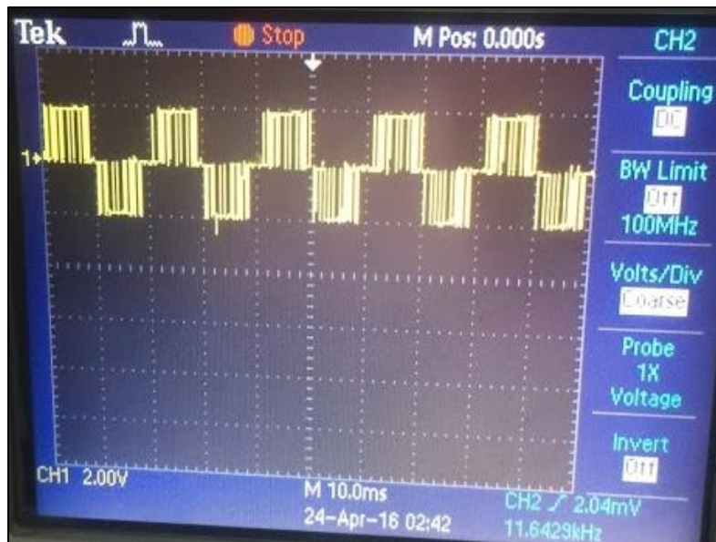
Figure 5.12. Inverter output voltage, V_{ab} .
