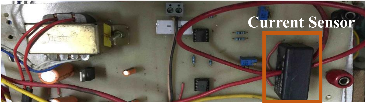
Figure 6.7: AC current sensor circuit
