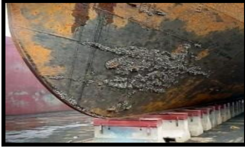
Fig 4.9 Corroded ship's hull[59]
