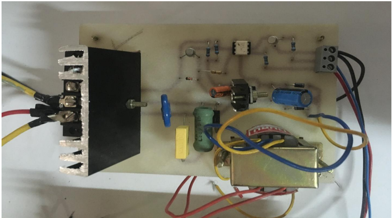
Figure 6.4 Switch unit of inverter
