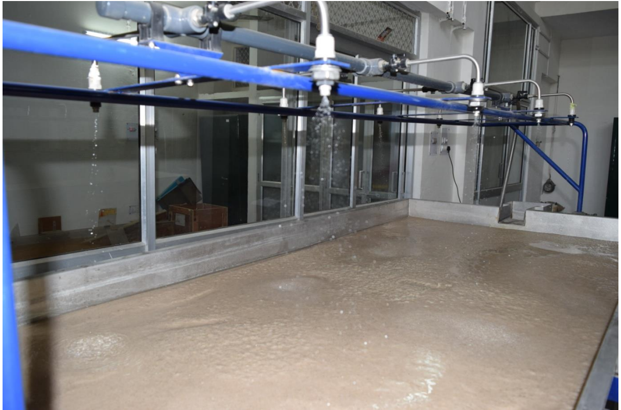
Figure 3.5 Eight spray nozzles for generating rainfall over the catchment area
