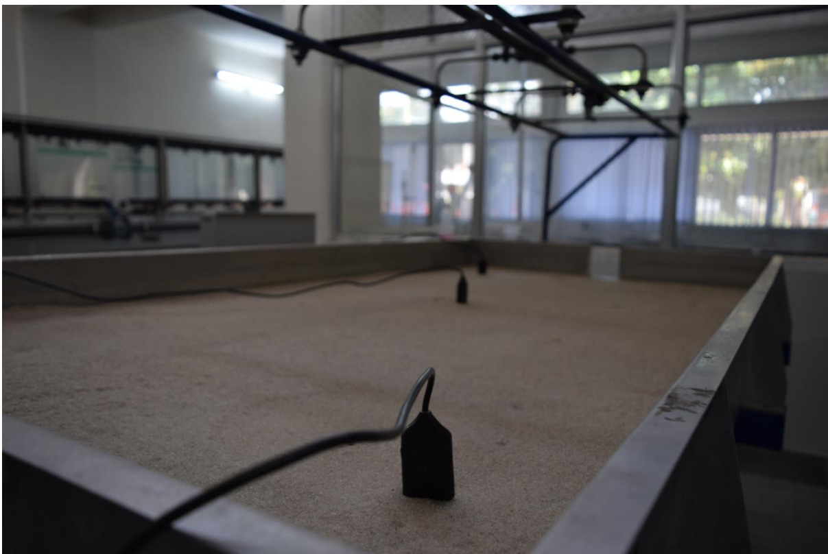
Figure 3.4 Soil moisture sensors for measuring antecedent soil moisture content
