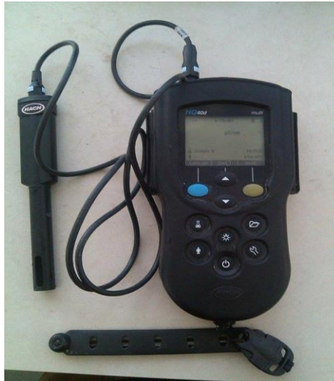
Fig. 3.4 Conductivity meter used for measurement of saltwater concentration
