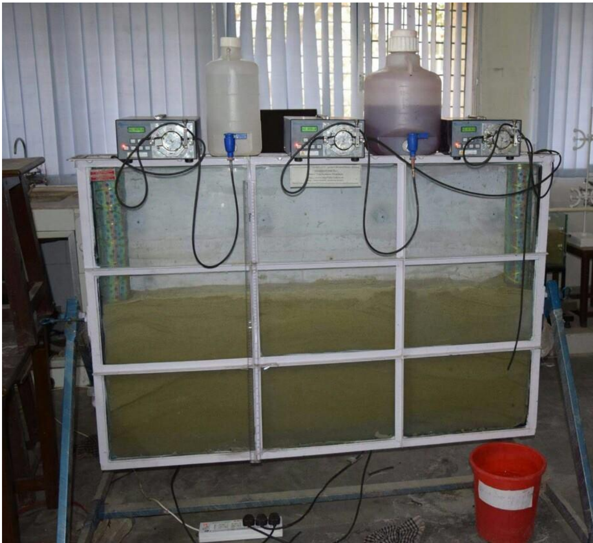
Fig 3.2 Experimental set up for investigating the dynamics of saltwater intrusion
