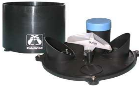
Figure 3.6. Rain wise tipping bucket rain gauge.
