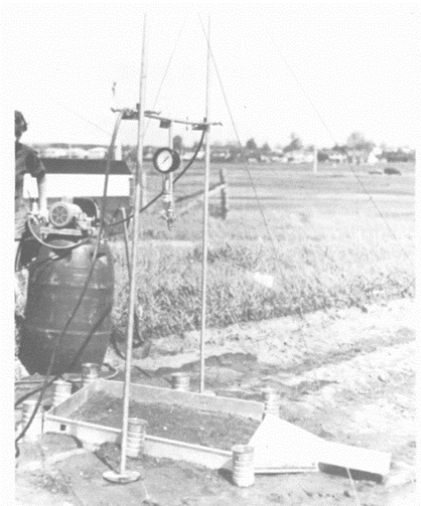
Figure 2.2. Photograph of Guelph rainfall simulator in the field. source; Canadian Agriculture Engineering Vol.29 No.2 summer 1987.
