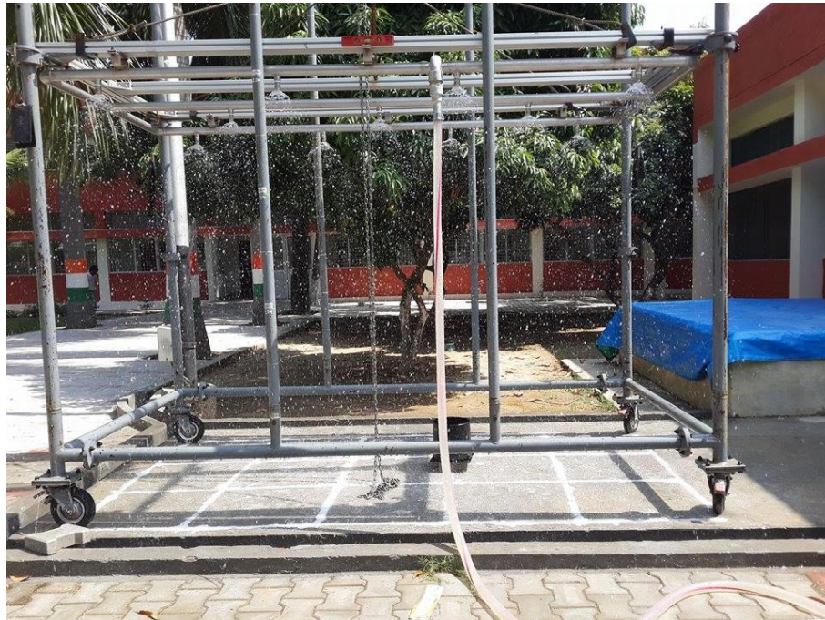
Figure 3.1. Rainfall simulator at Department of Hydrology IIT Roorkee.
