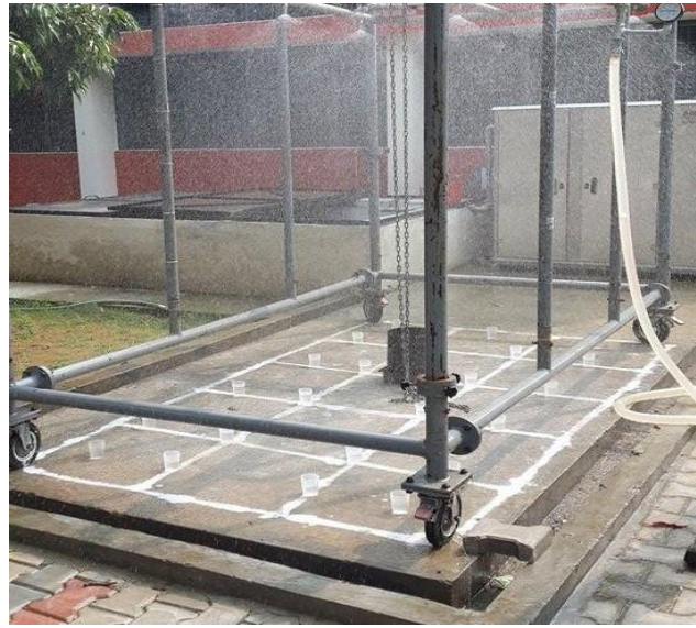
Figure 3.5. Water collecting beakers in array for CU estimation.
