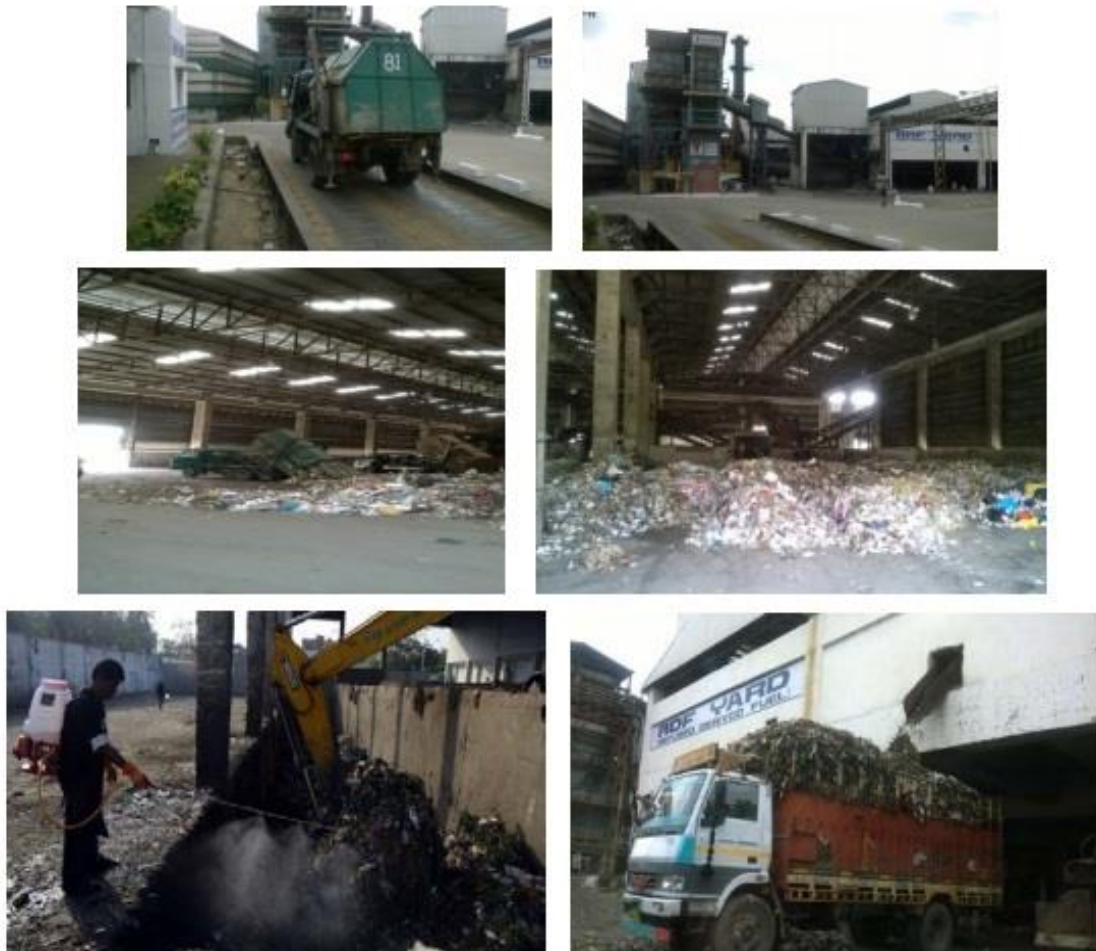
Figure 4.7: Processing of Solid Waste at refuse derived fuel plant in Chandigarh
