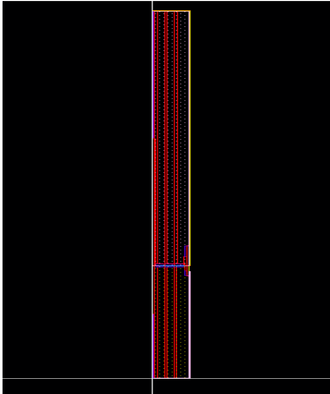
Fig. 4.14 Layout for n_f (non-uniform) = 1 (controlling MOS) and 9 (driving MOS).
