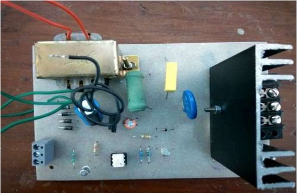
MOSFET switch with its driver circuit
