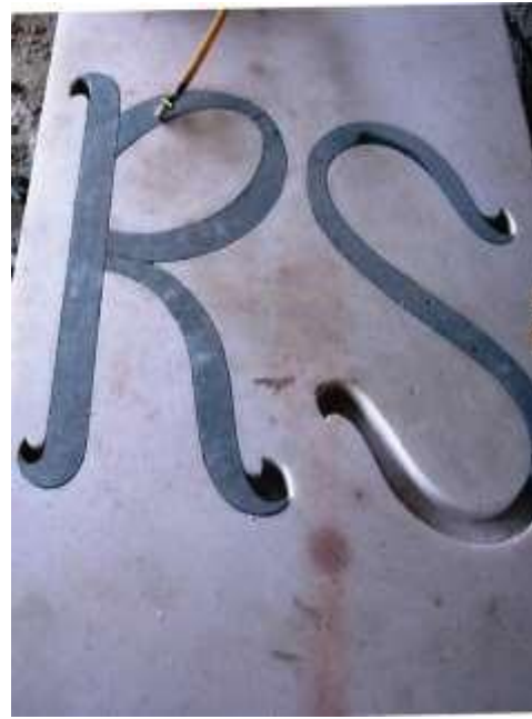
Fig 3.7 Fixing of coloured stone
