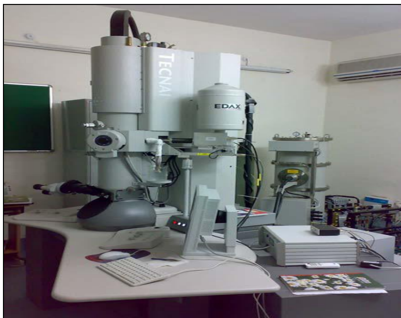
Figure 2.11: Photograph of 200 KeV FEI Tecnai G 2 TEM at Institute Instrumentation Centre, Indian Institute of Technology, Roorkee.
