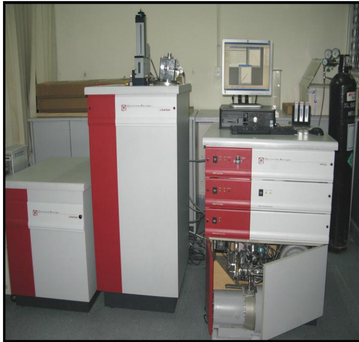
Figure 2.19: Schematic diagram of SQUID magnetometer.
