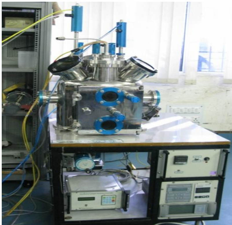
Figure 2.4: Magnetron Sputtering System.
