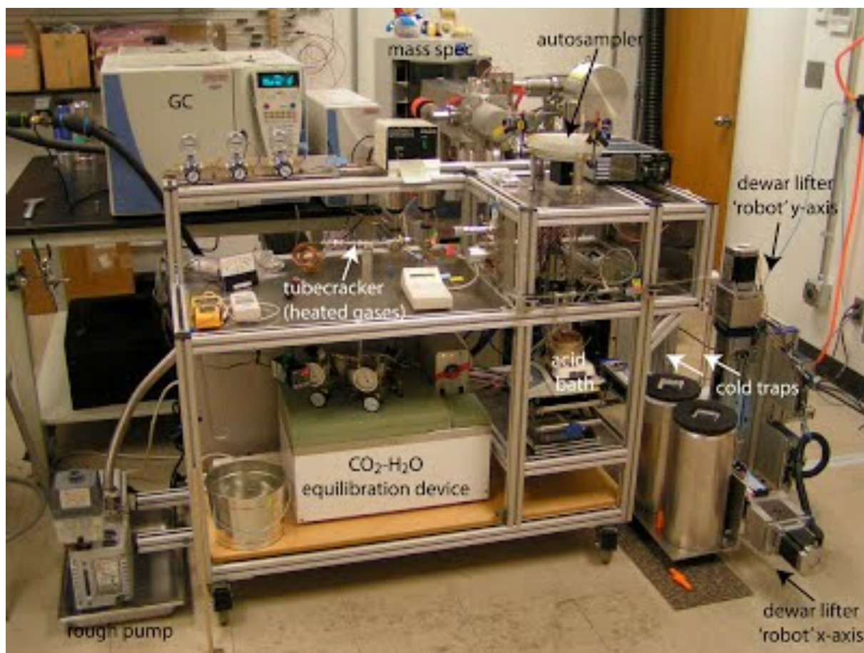
Figure 4.5 Autoline for clumped isotope analysis (Johns Hopkins University)
