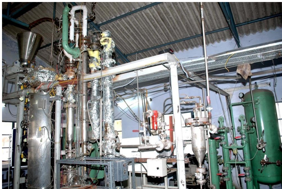
Figure 3.1b: Experimental setup of fluidized bed pyrolyzer
