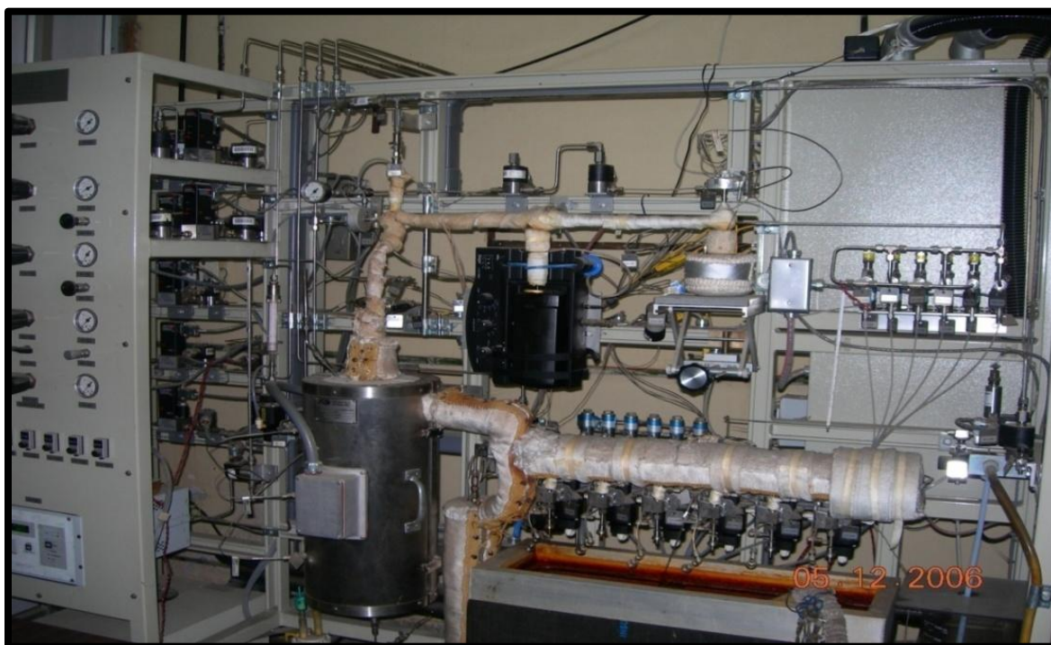
Figure 3.2b: Experimental setup of advanced cracking evaluation (ACE-R) FCC unit
