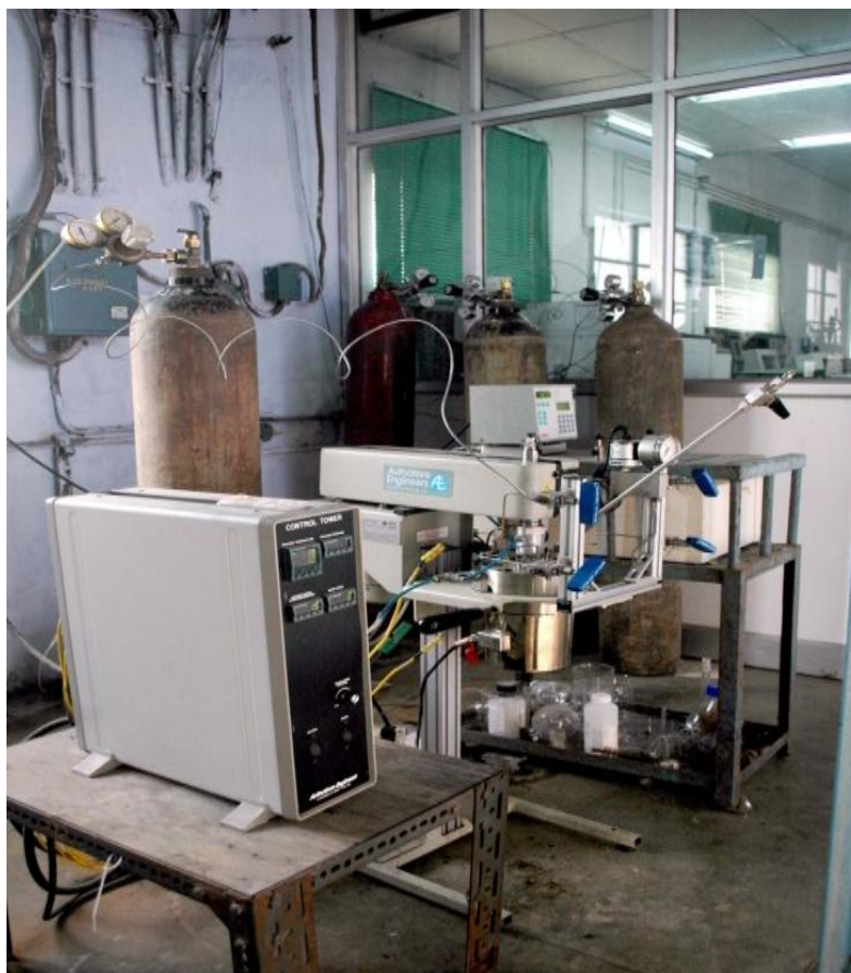
Figure 3.3b: Experimental setup of CSTR
