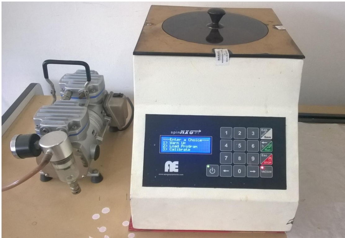
Figure 4.5.2 Spin NXG spin coating equipment with vacuum pump
