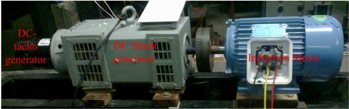
Fig. A 3.5 Induction Motor Coupled with DC-Shunt generator and Tacho-generator
