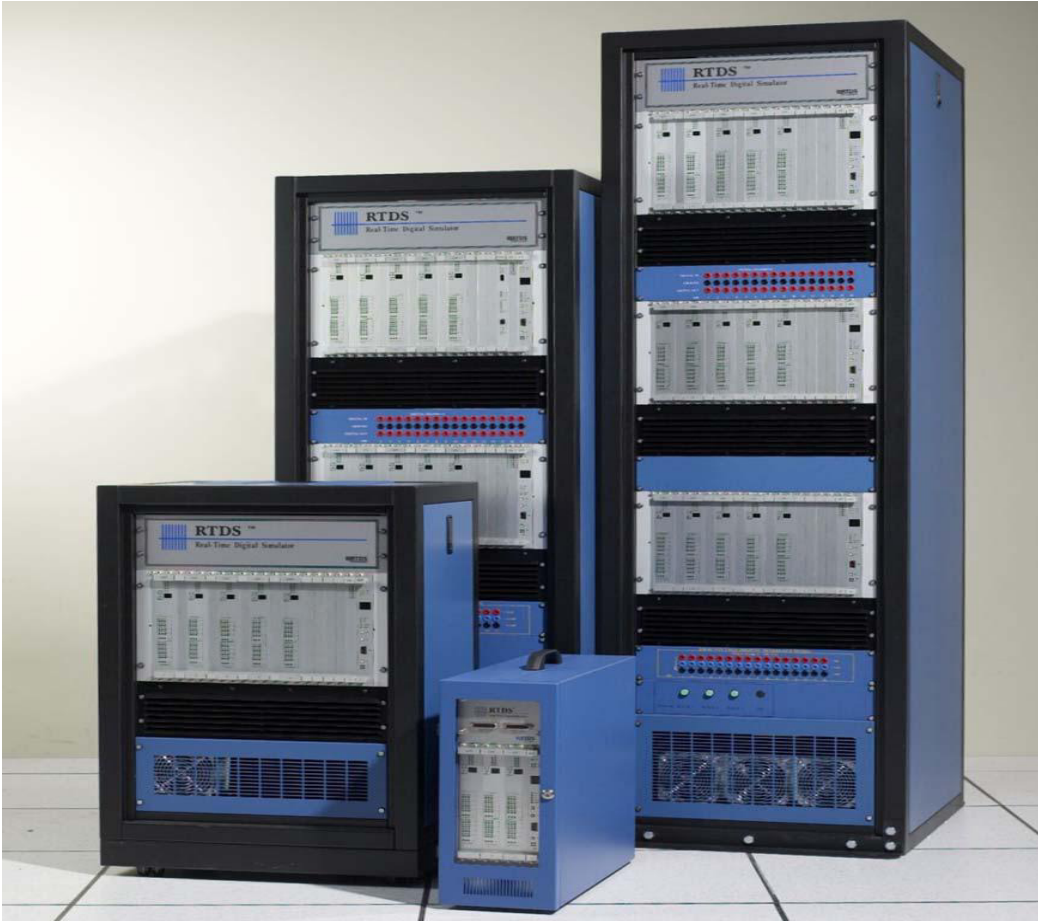
Figure i: Real-time Digital Simulator with Racks
