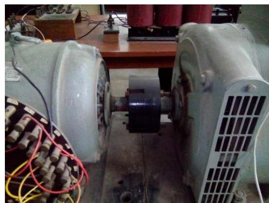
Fig. 7.1: Experimental set up showing (a) schematic diagram (b) general view (c) decoupled and (b) coupled test synchronous machine and DC machine.
