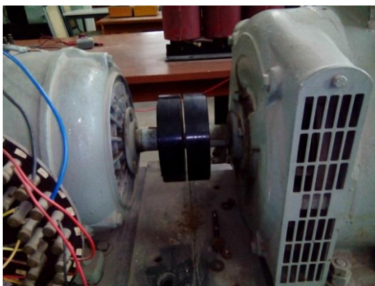
Fig. 7.1: Experimental set up showing (a) schematic diagram (b) general view (c) decoupled and (b) coupled test synchronous machine and DC machine.
