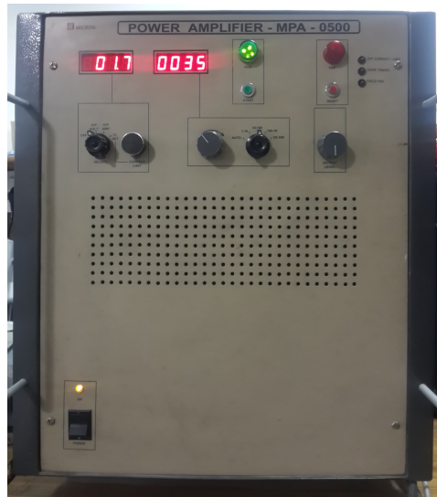
Fig. 3.12: Power amplifier to excite electrodynamic shaker at different frequencies
