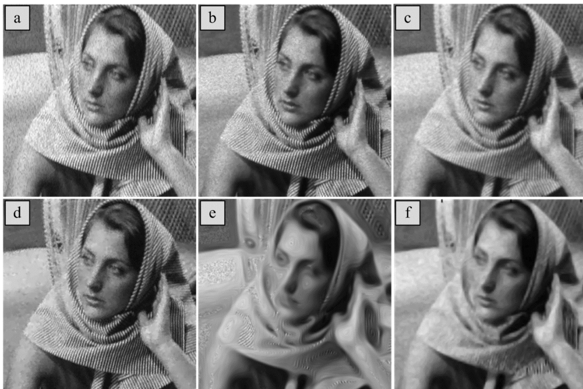
Figure 3.6 Visual quality comparison for iterative nonlinear filters: (a) DsFgf4d [29.02, 0.547, 24.38], (b) DsFsrاد [43.16, 0.73, 10.79], (c) DsFad [36.91, 0.66, 15.47], (d) DPAD [47.63, 0.76, 8.34], (e) CED [36.16, 0.54, 16.14], (f) Level set [32.45, 0.39, 20.01] whereas the noisy image [40.06, 0.652, 12.09]
