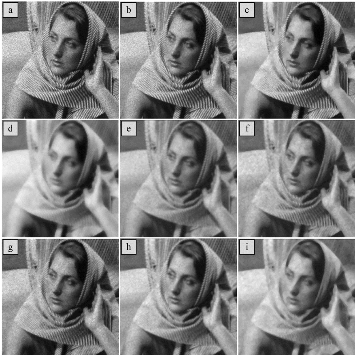
Figure 3.5 Visual quality comparison for variational and nonlinear filters: (a) AFTV [41.45,0.67, 11.71], (b) ROF [45.87, 0.72, 9.24], (c) ATV [43.21, 0.65, 10.76], (d) Aujol et al. [17.18, 0.1, 48.16], (e) Shock [35.53,0.56, 16.75], (f) Median [33.98,0.46, 18.30], (g) DsFhmedian [40.05, 0.63,12.91], (h) DsFhomog [37.44,0.6, 15.0], (i) DsFhomo [35.4, 0.49, 16.87 ] whereas the noisy image [40.06, 0.652, 12.09]
