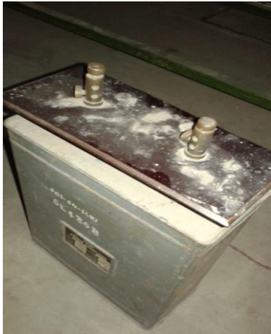
Fig. 4 Ac power capacitor
