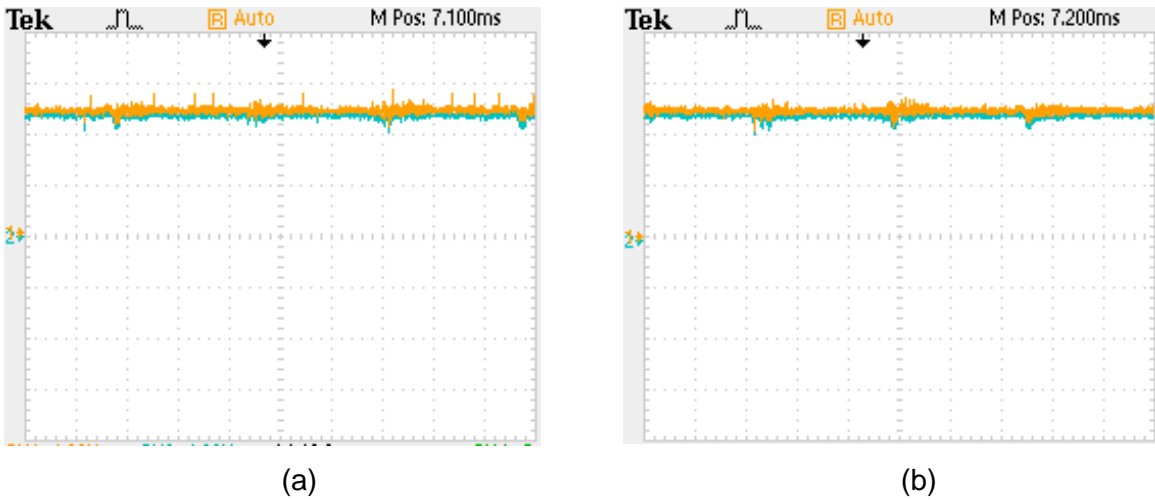
Fig. 3.27: a) dc capacitors voltages PI controller (b) dc capacitors voltages with T2FLC
