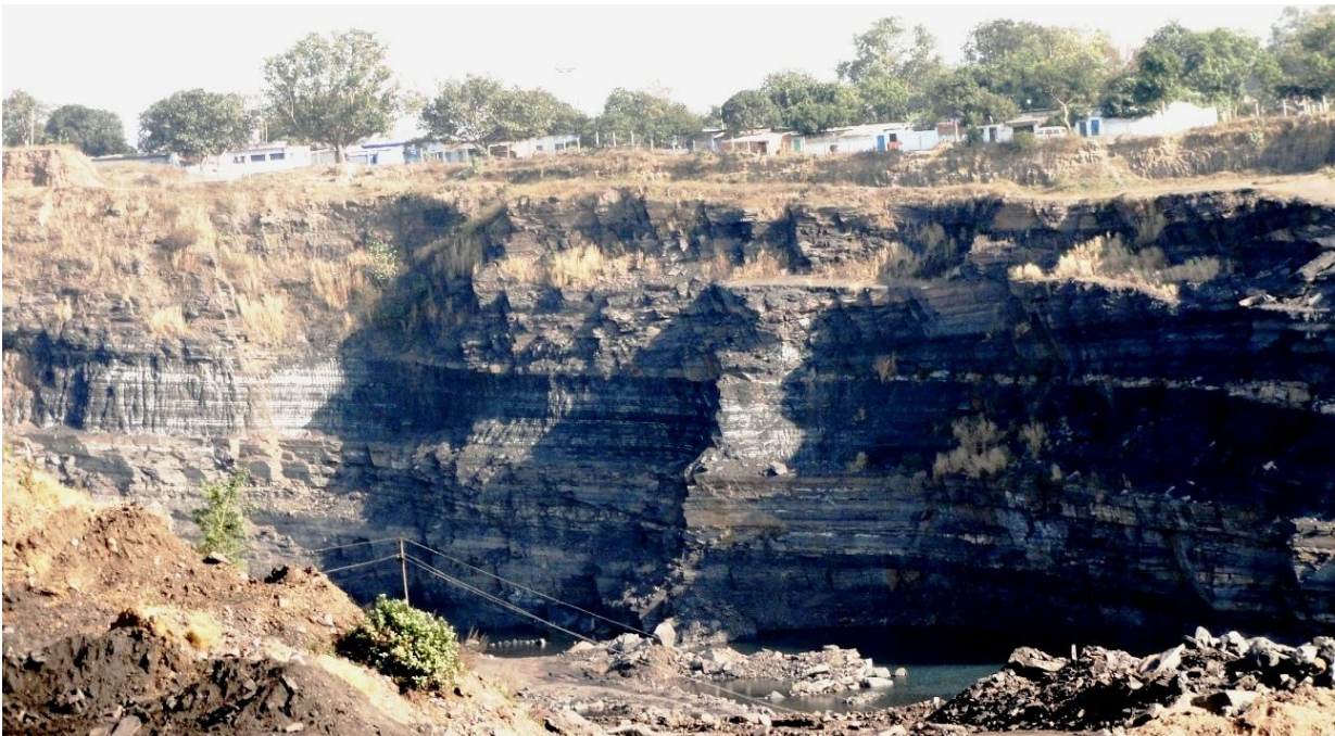
Figure 3.4 Alternate bands of almost horizontal dipping sandstone and shale exposed due to mining near Sonardh, area, JCF
