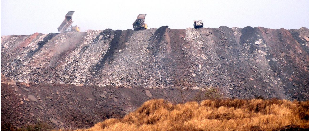
Figure 3.10 Massive overburden of waste mine material dumped in and around Alkusa colliery, JCF. The overburden dump also has a lot of carbonaceous material that can catch fire (Prakash et al., 2013)
