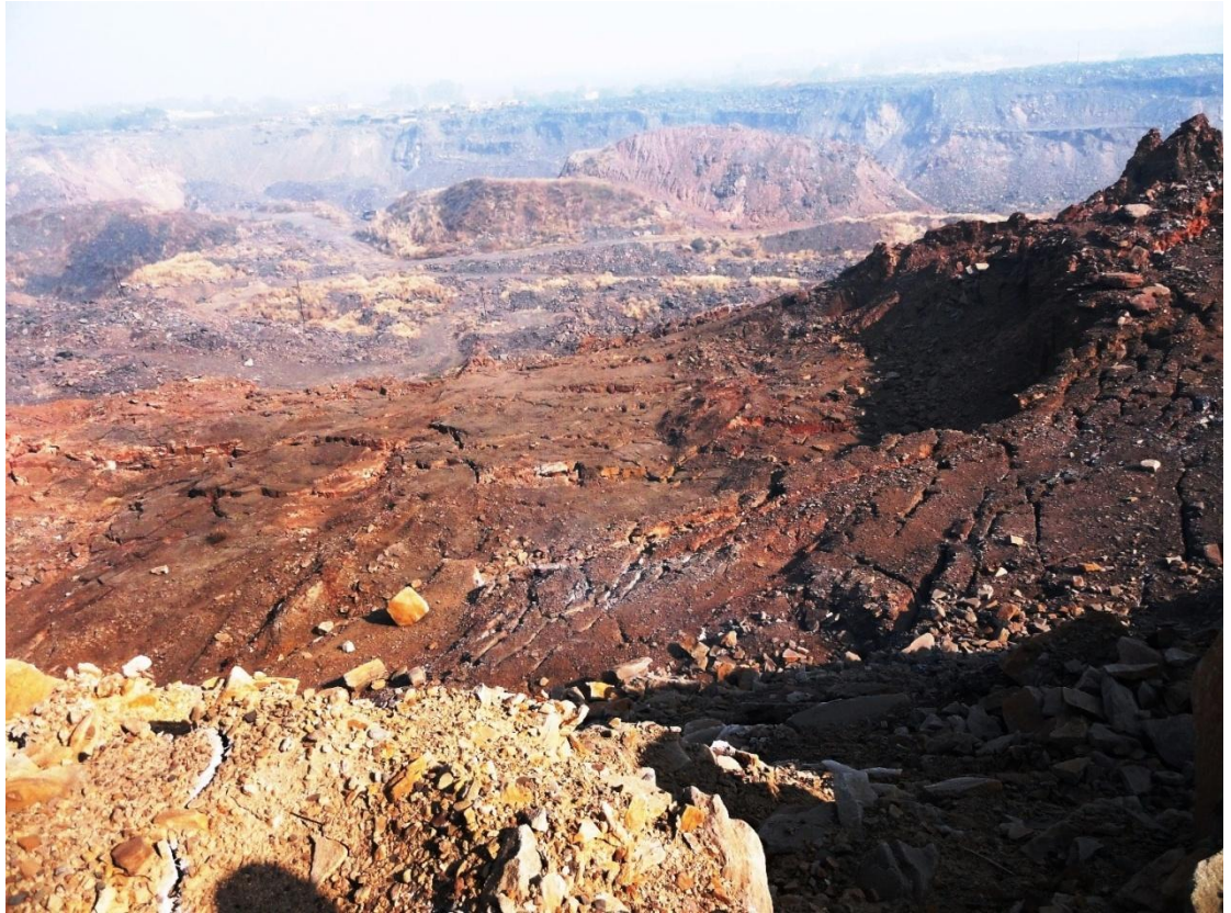
Figure 3.12 Rugged landscapes in the Bokapahari area, JCF, due to mining and coal fire-induced uncontrolled subsidence. The surface contains fissures of all dimensions. This photograph was taken looking south (Prakash et al., 2013)
