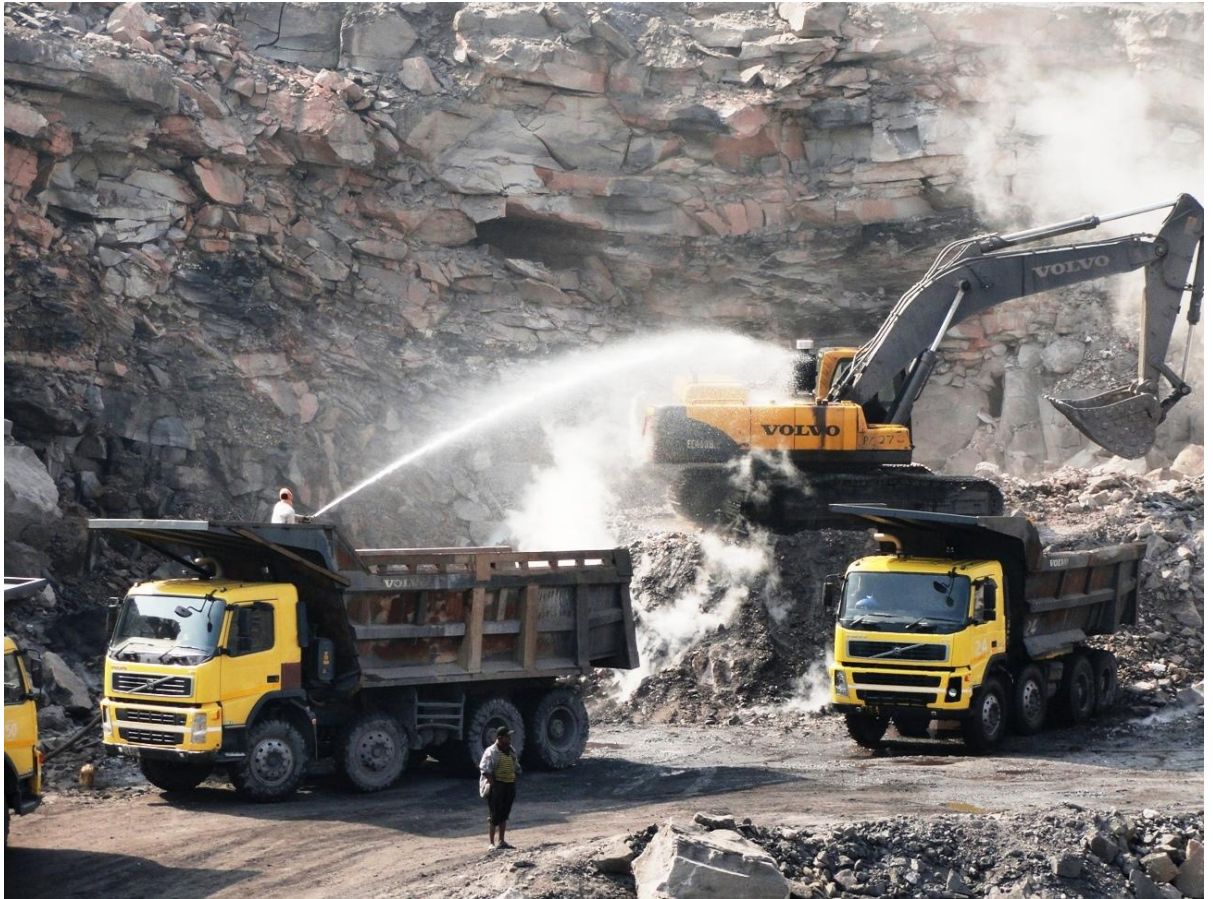
Figure 3.7 Coal extraction in the Sijua opencast mine in the JCF. Dousing the fire with water, excavating the burning seam and using the unburnt coal are popular means of keeping the coal fire under control (Prakash et al., 2013)
