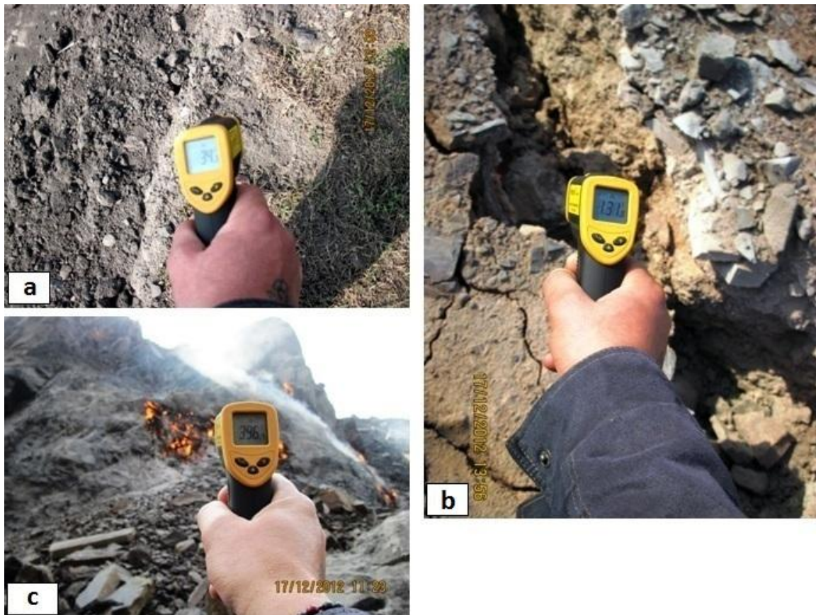
Figure 3.13(a)-(c) Temperature measurements using a portable field thermometer in the field (a) showing 34°C temperature on the surface, (b) 131°C temperature of smoldering fire in the crack (c) 396°C temperature of a burning coal seam (measured from approximately 30 m distance) (Photo courtesy by Ms. Varinder Saini, December, 2012)
