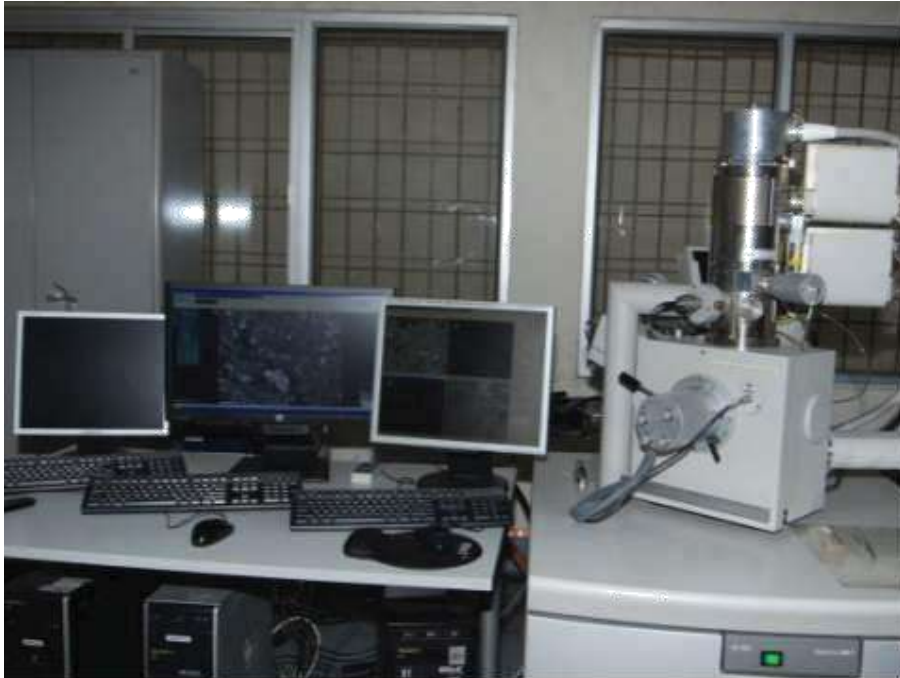
Figure 3.5: The Photograph of FEI Quanta 200 FEG-SEM.
