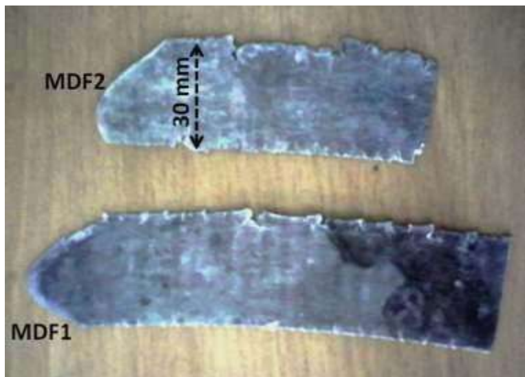
Figure 7.3: Photograph of UFG alloy sheets obtained through MDF1 and MDF2 routes.
