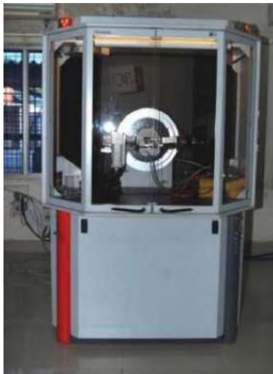
Figure 3.8: Photograph of the XRD unit /2 (Bruker AXS D8 Advance diffractometer)
