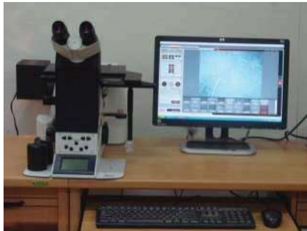
Figure 3.4: The Photograph of LEICA DMI5000 M optical microscope.
