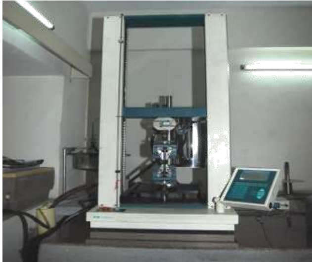
Figure 3.12: The photograph of the S-Series, H25K-S tensile testing machine.
