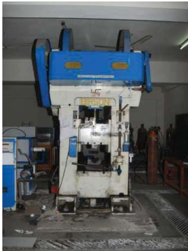
Figure 3.3: Friction screw forging press used for cryoforging
