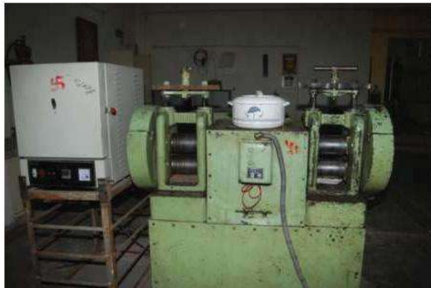
Figure 3.1: Schematic of experimental setup for cryorolling.
