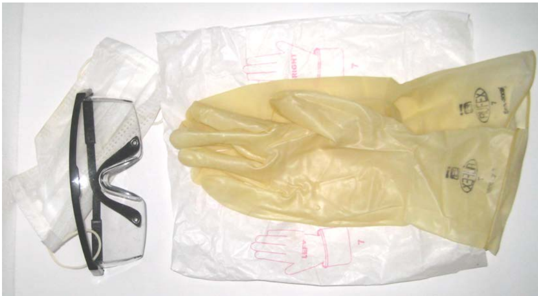
Fig 3-34 Items to be used strictly when working with nanomaterials (Mask, Glass & gloves)
