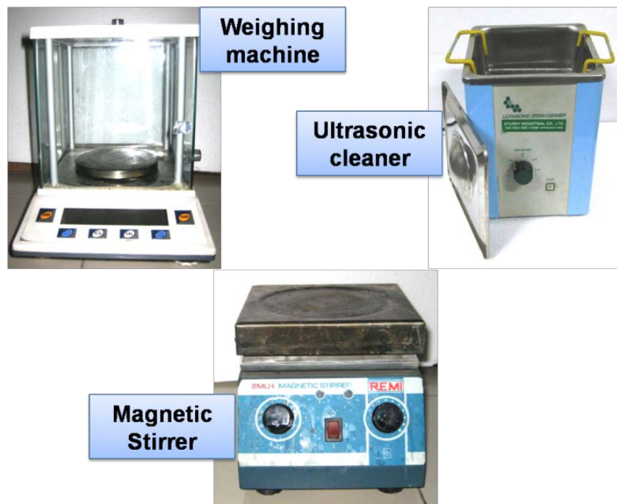
Fig 3-9 Auxiliary devices used in present study; digital weighting balance, ultrasonic cleaner and magnetic stirrer
