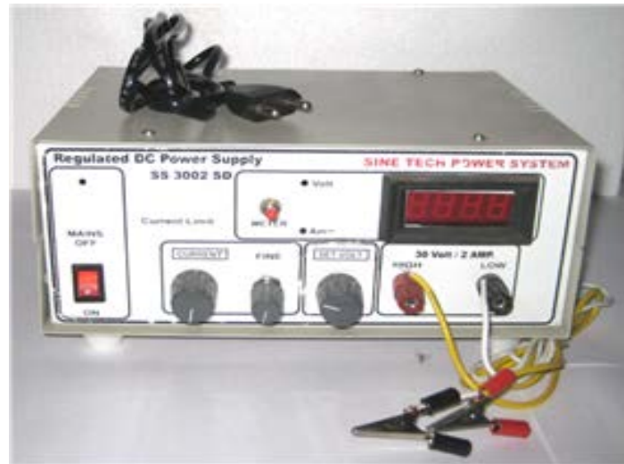
Fig 3-8 Regulated DC power supply used as a potential source during coating process Other supplementary devices partially used in the present investigation are digital weighting balance, ultrasonic cleaner and magnetic stirrer as shown in Fig 3-9.
