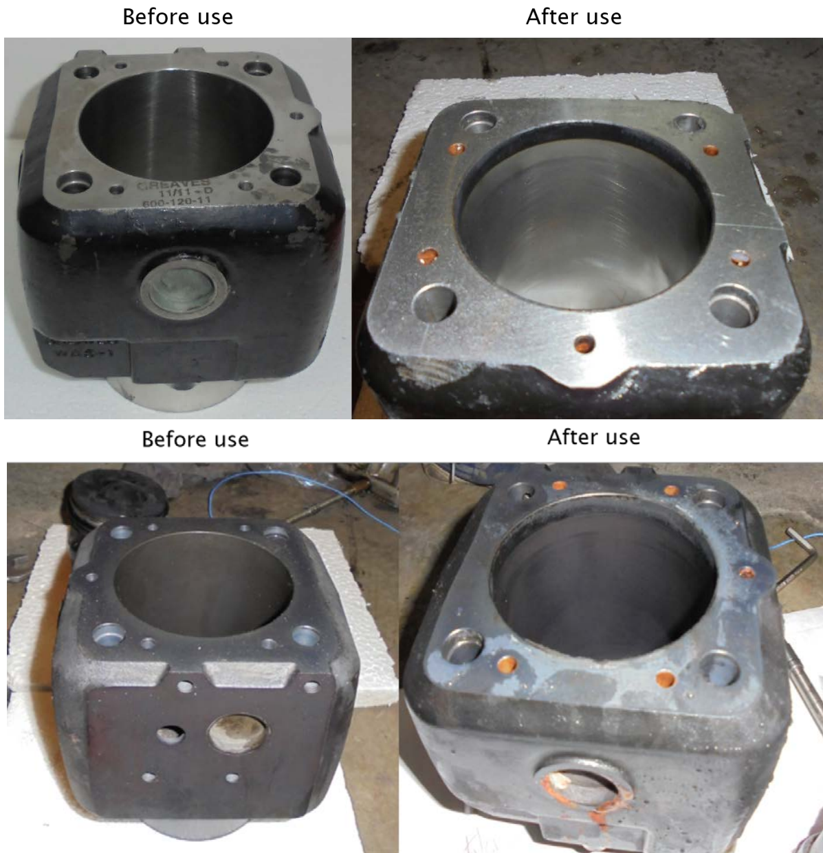
Fig 4-36 Pictures of engine blocks before and after use; uncoated (top right and left) and coated (bottom right and left)
