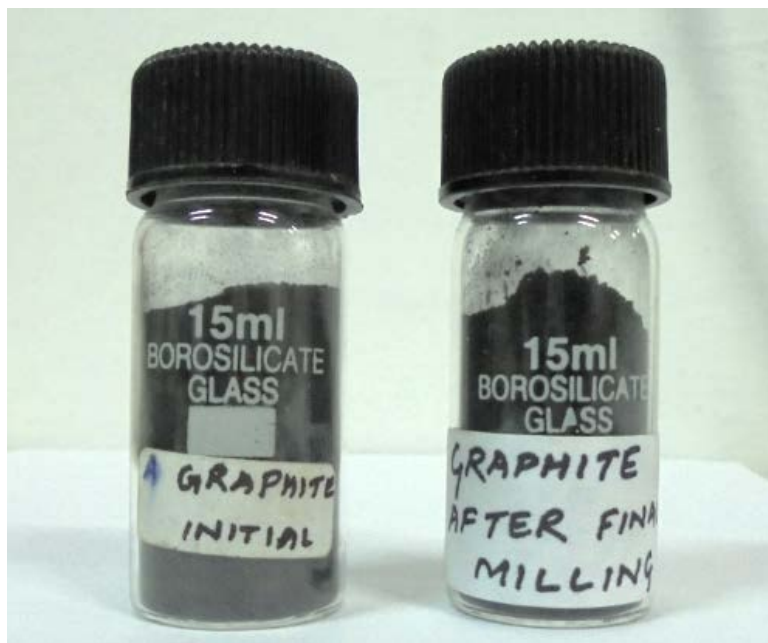
Fig 4-2 Graphite powder in container; before and after milling
