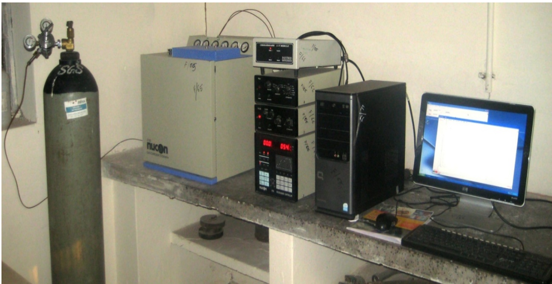
Fig 3-40 Gas chromatograph experimental set-up
