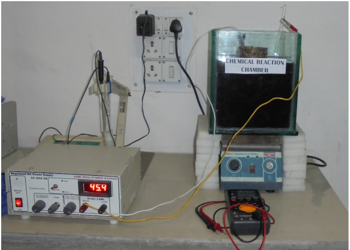
Fig 4-35 Photograph of real time coating experiment of engine block; showing DC supply (~45 V) connection to work and counter electrode in electrochemical cell
