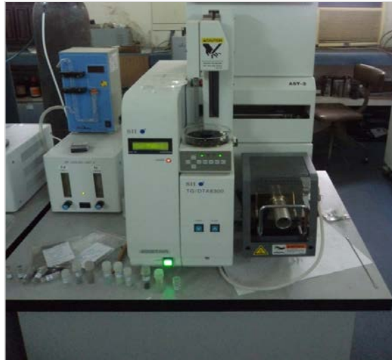
Fig 3-32 A photograph of TGA system used to measure thermal stability of the samples under various conditions of temperature and environment
