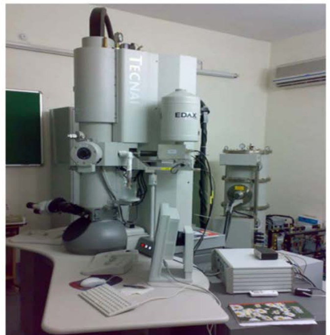
Fig 3-28 A ray diagram of TEM in image mode and photograph of FEI Tecnai-20 TEM
