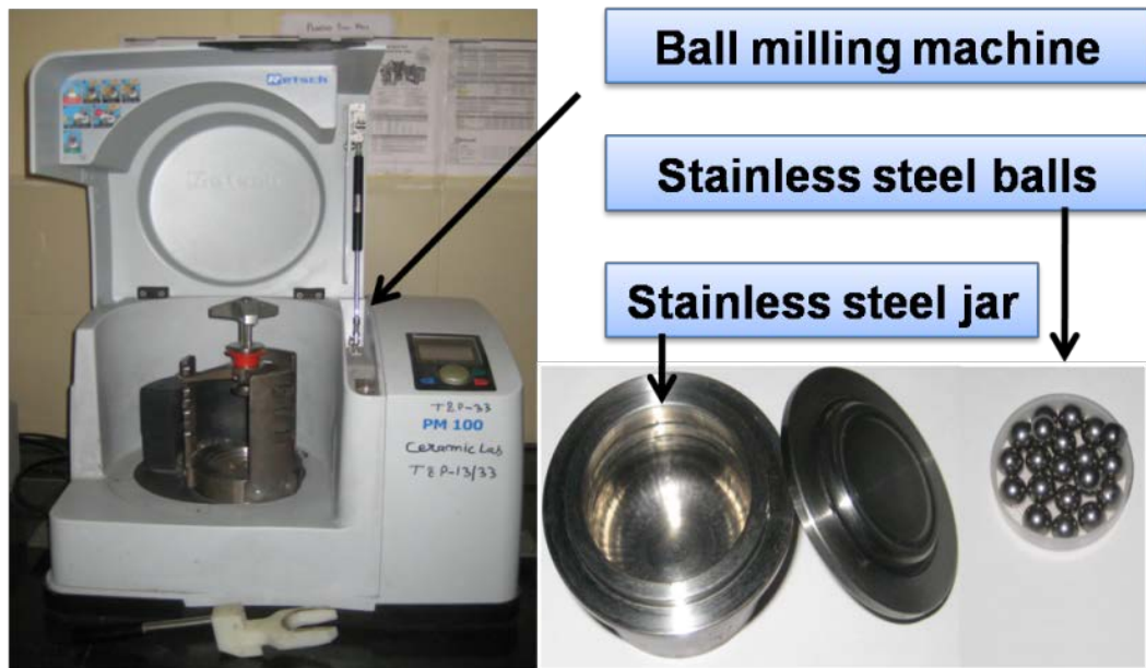
Fig 3-5 Planetary ball milling machine (Retch, Model PM100) used for graphite nanoparticle synthesis
