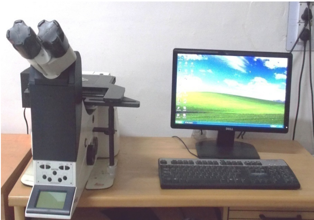
Fig 3-27 Optical microscope (Lieca) used for examination of sample microstructure
