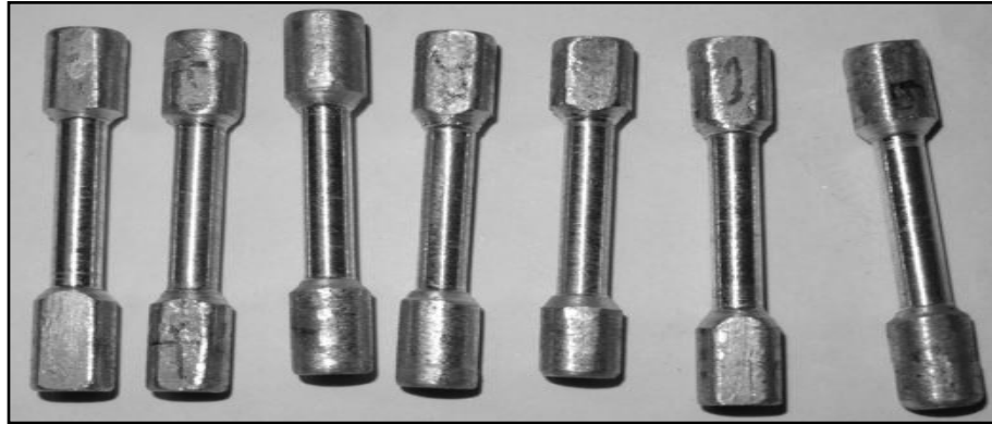
Fig. 4.5 Tensile test pieces machined from hot forged samples
