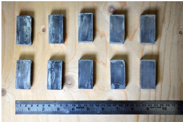
Fig. 4.4 Samples after hot forging
