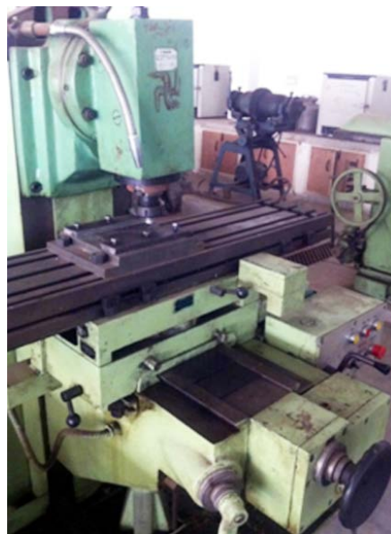
Fig. 3.2: Vertical milling machine used for FSP experiments
