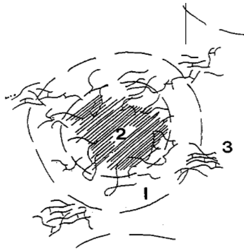
Fig. 2.10: Schematic structure of NCGPEs where 1 represents the highly conductive interface layers coating the surfaces of grains, 2 represents the dispersed insulating grains and 3 represents the matrix polymer ionic conductor. (Wieczorek et al, 1994).
