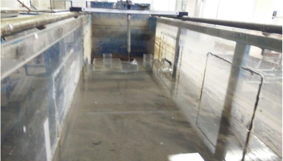
Figure 8.7: Fusegate working under Normal Condition
