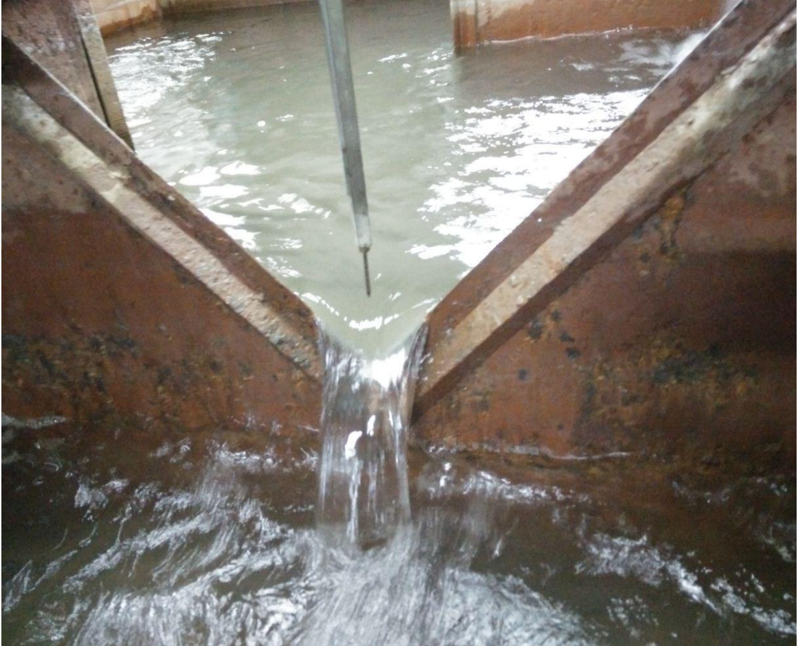
Figure 8.1 Discharge measuring device (V-Notch) in laboratory
