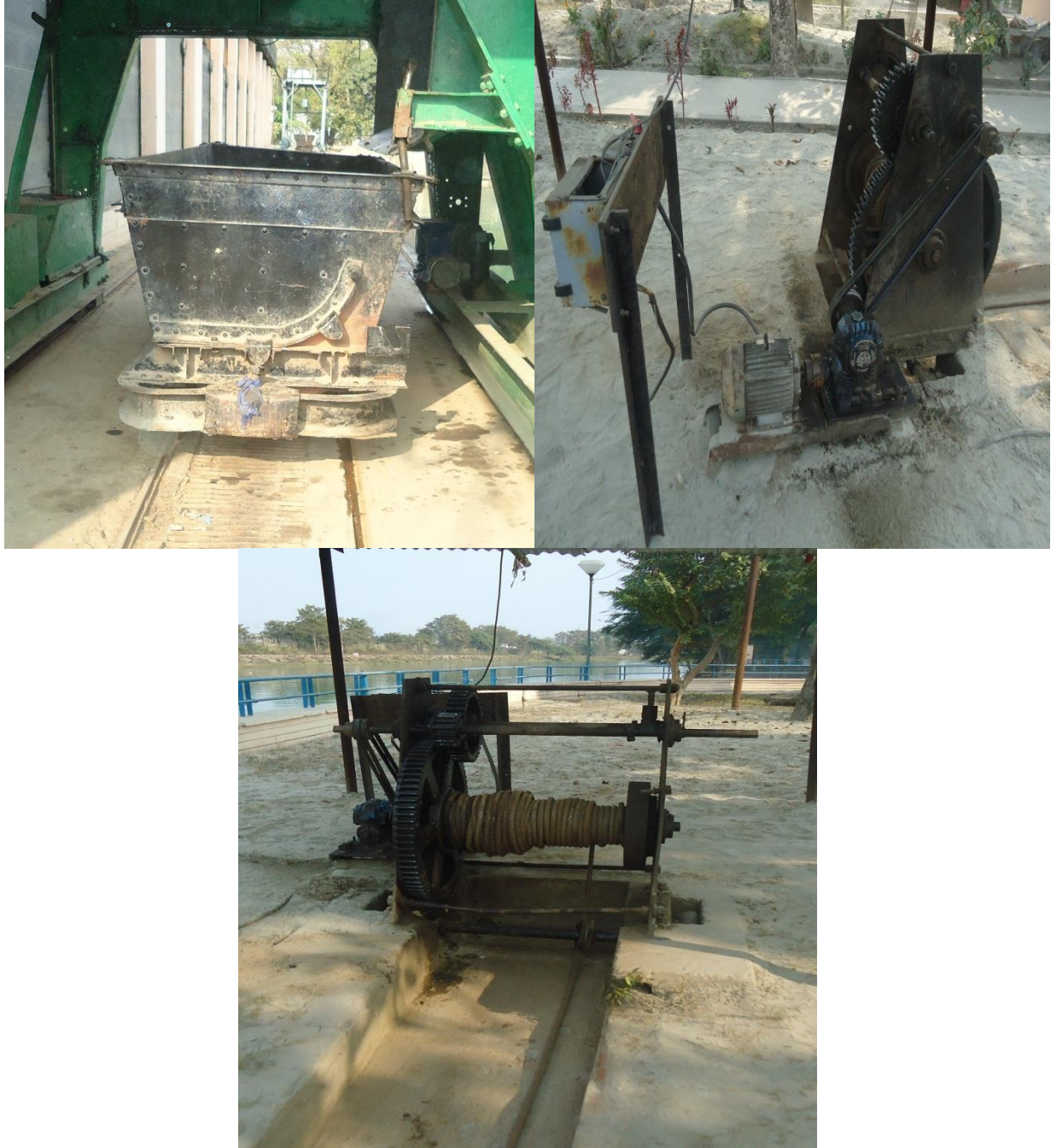
Fig 4.12:-Trash Trolley And Pulley Arrangement To Disposed The Trash
