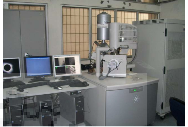
(b) Fe-SEM QUANTA 200 FEG (FEI Netherlands)
