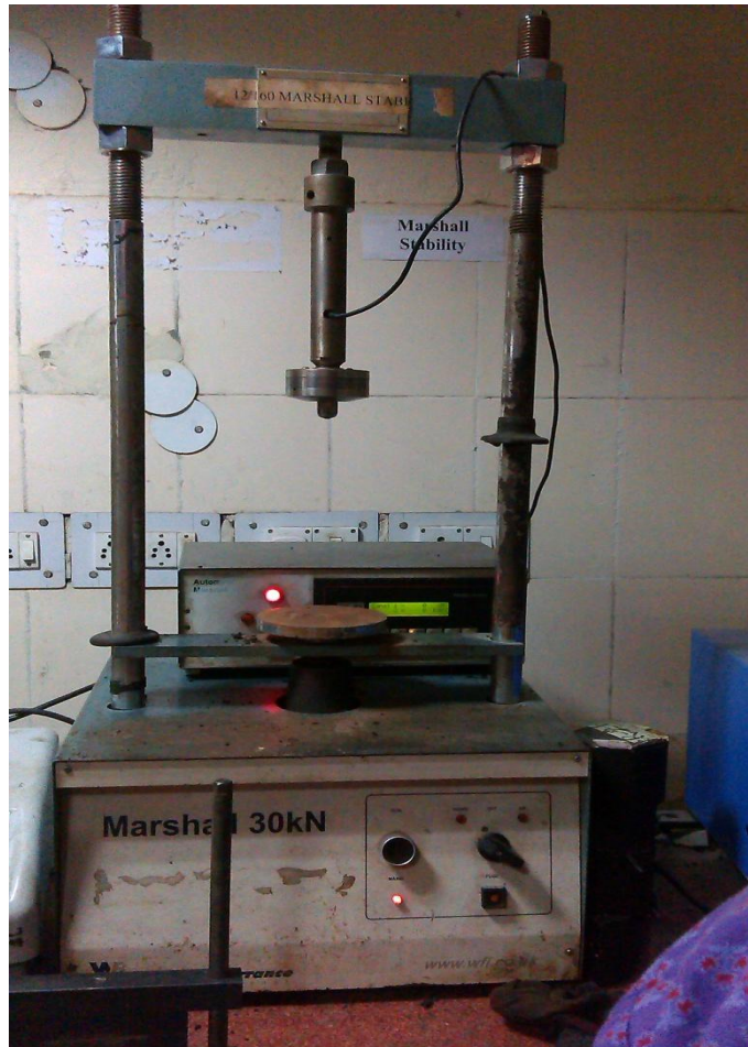
Figure 3.11: Marshall Setup for ITS Test
