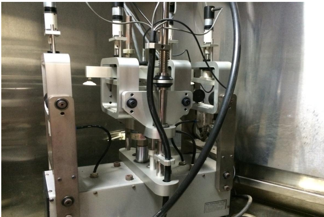
Figure 3.20: Four point Bending Beam Apparatus inside UTM
