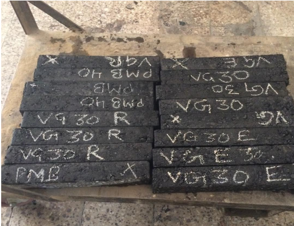
Figure 3.19: Beams prepared using automatic slab roller compactor
