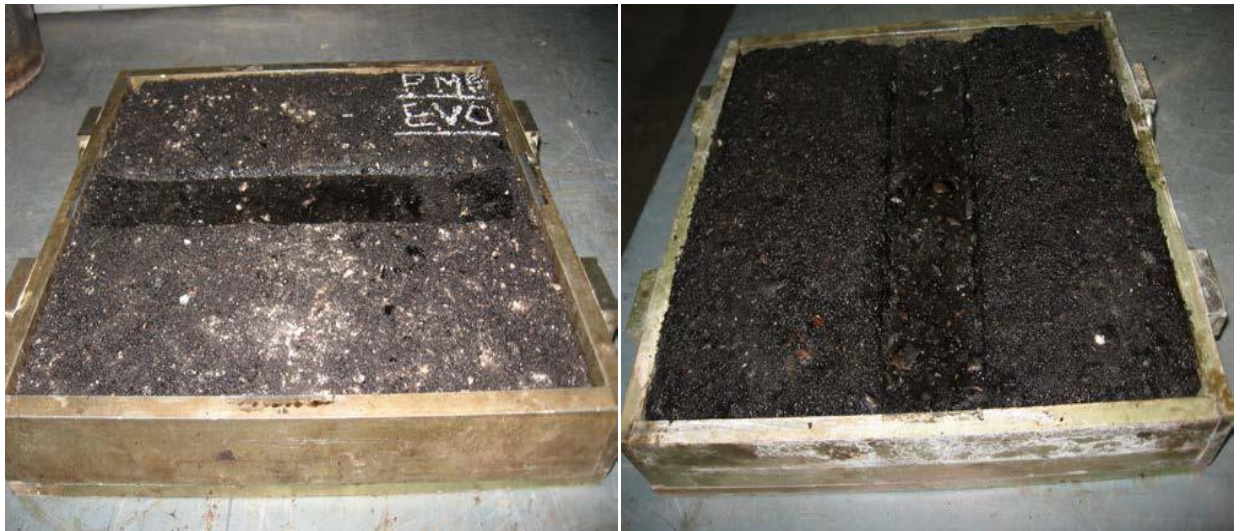
Figure 3.21: Wheel Rutting Test Samples
