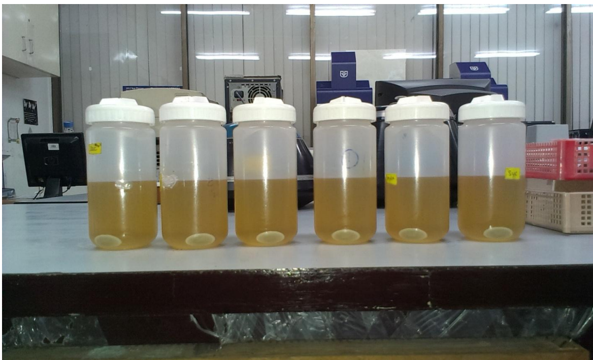
Figure 5.4.6: The bottles containing Mother Liquor as shown above and crude Biosurfactant after centrifugation
