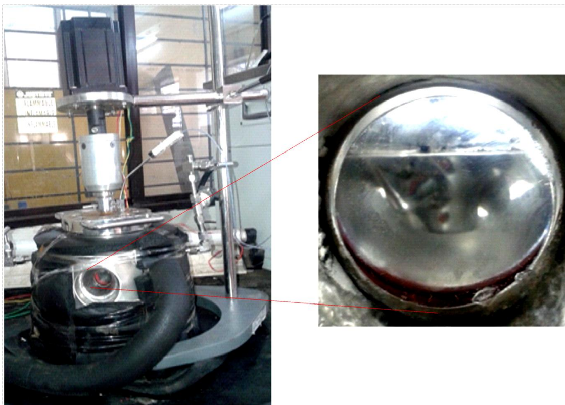
Figure 4.2.3: Experiment set up of Stirred Tank Reactor (STR) Along with Transparent Window used in present study
