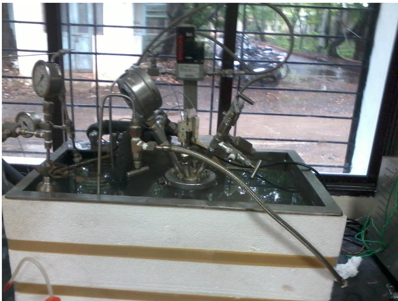
Figure 4.1.2: Experimental Setup to Study the Effects of Zeolite 5A, Zeolite 13X, Silica Sand on CO 2 Hydrate Formation
