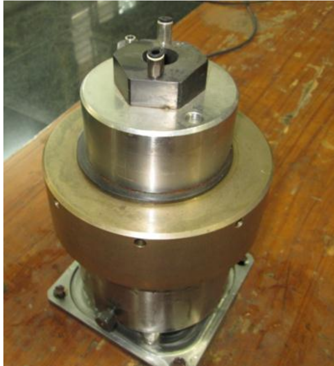
Figure 4.4.3: Hydrate Cell in Close Condition
