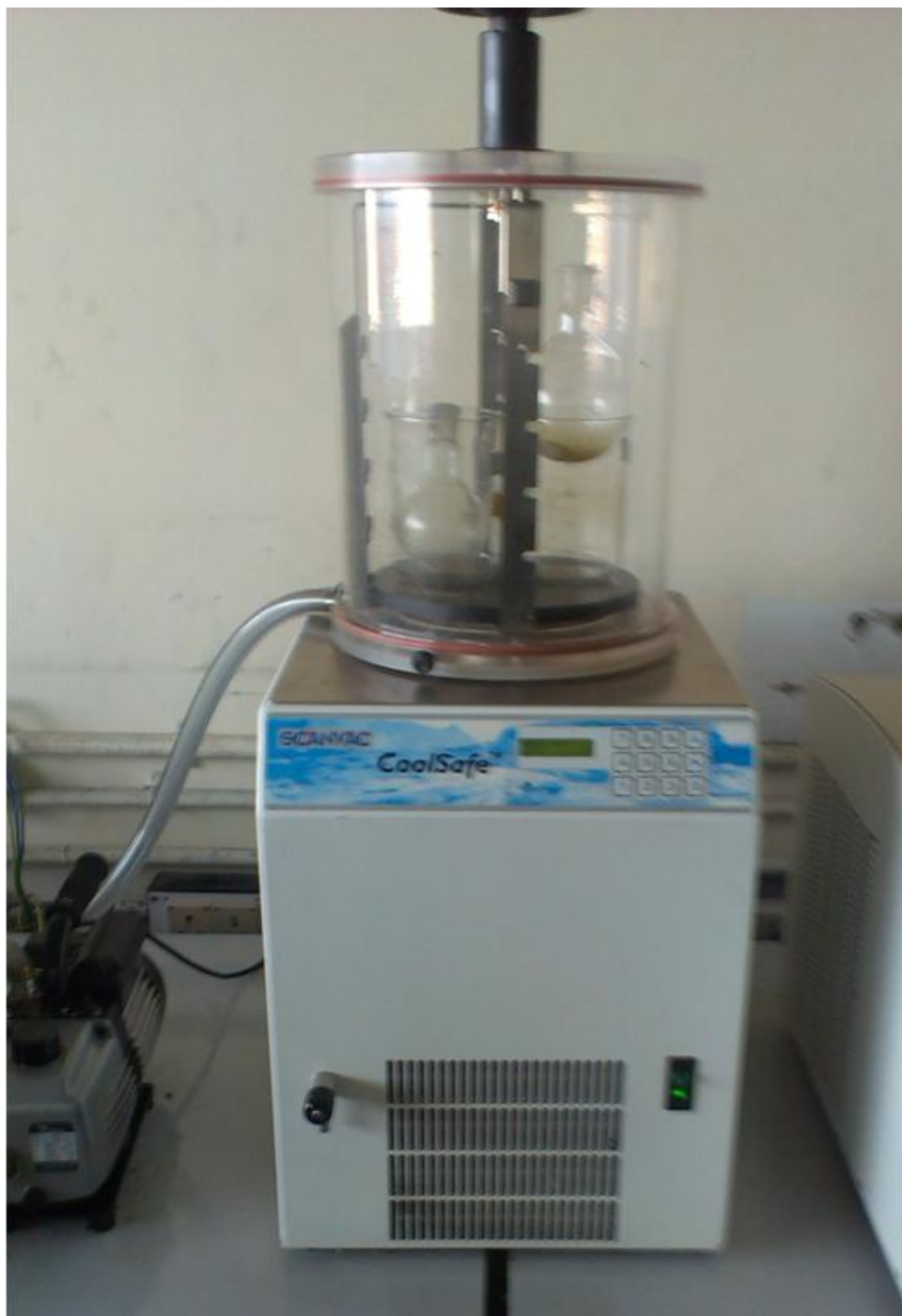
Figure 5.4.8: Lyophilizer used for Lyophilization of Biosurfactants
