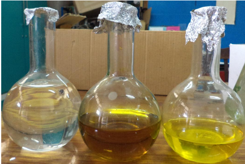
Figure 5.5: Colouring agents used for phenol and cyanide analysis Nickel Solution (left) Potassium ferricyanide (centre) and picric acid solution (right)
