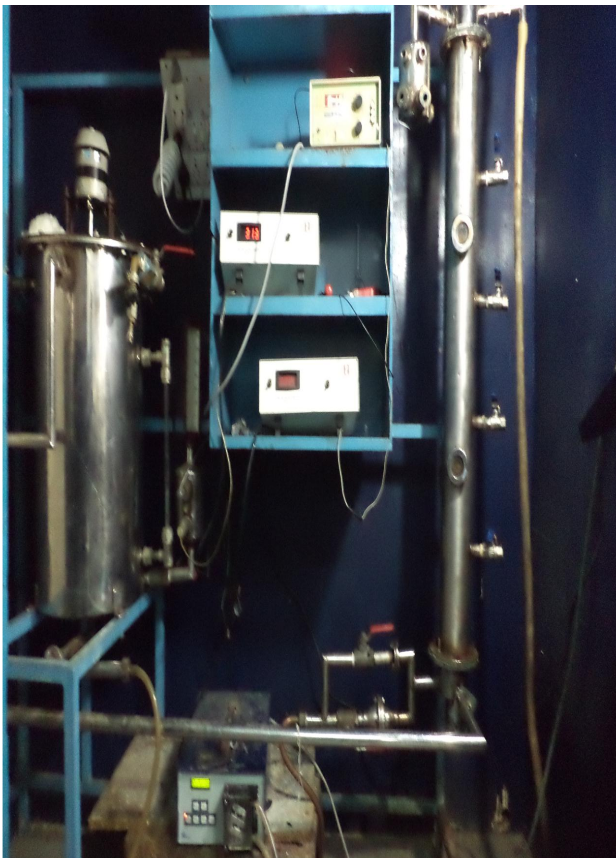
Figure 4.4 Complete reactor setup for column studies
