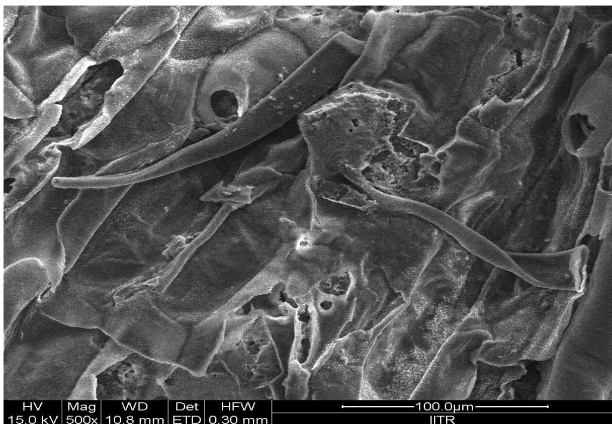
Figure 6.19: SEM images of corn husk leaves with immobilised bacteria after SAB of phenol and cyanide
