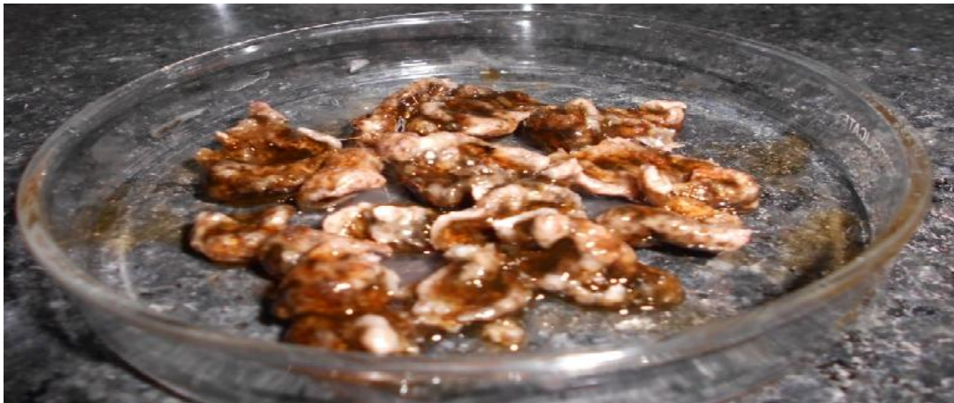
Fig:4.1 Sulfonated Polystyrene Resins using acetone(SPR-2)
