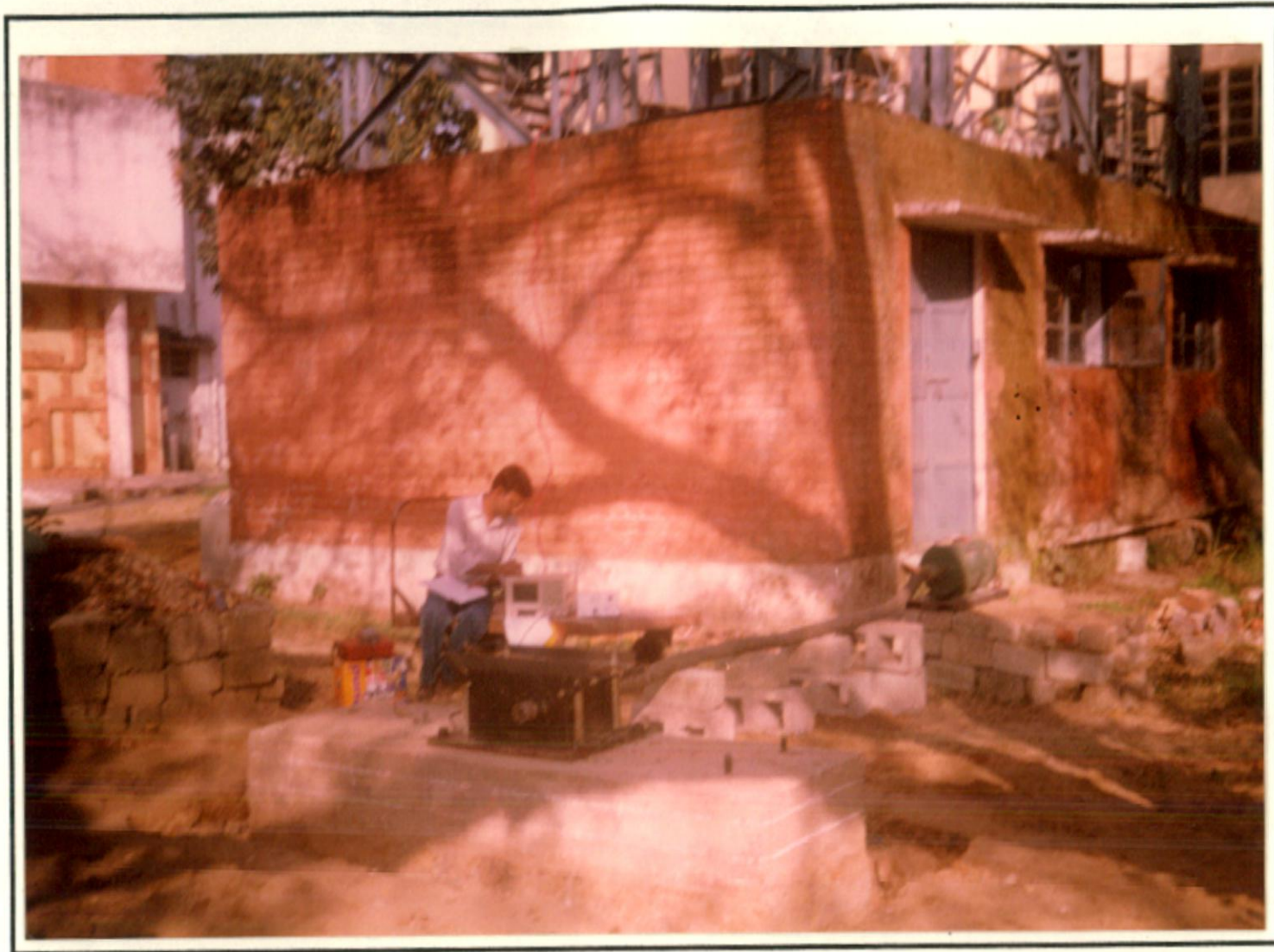
Fig. 17 Vertical vibration test with the oscillator at the centre of the block
