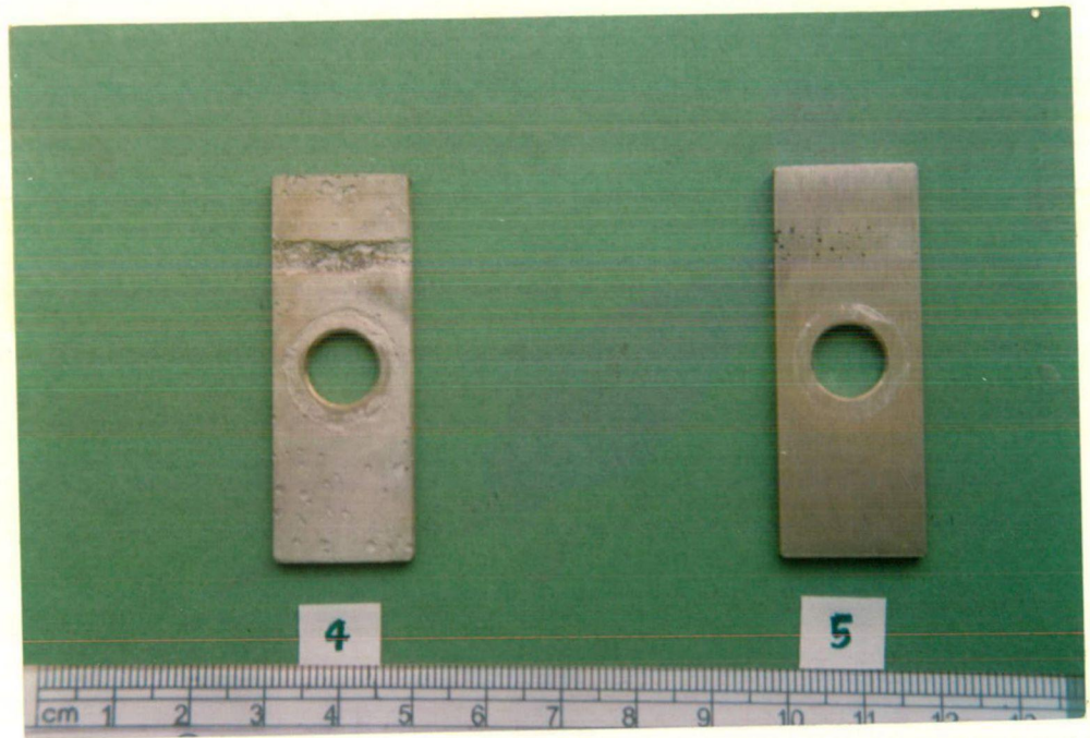
Fig. 3.6 : CORRODED COUPONS OF 2205 (NO.4) AND 254 SMO (NO.5) MILL A (C-WASHER, GASEOUS PHASE)
