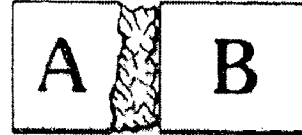
(b) GALVANIC CORROSION
