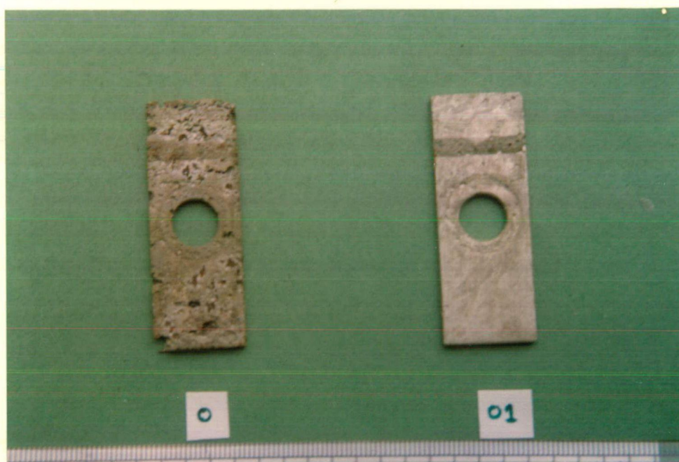
Fig. 3.4 : CORRODED (NO.2) AND FRESH (NO.1) COUPONS OF SS 316L MILL A (C-WASHER, GASEOUS PHASE)
