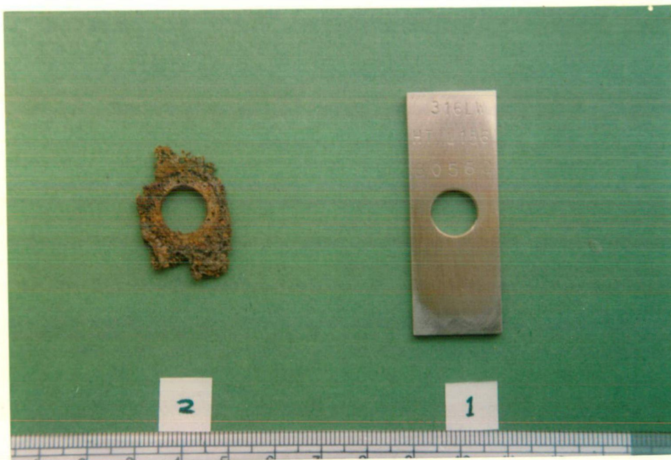
Fig. 3.4 : CORRODED (NO.2) AND FRESH (NO.1) COUPONS OF SS 316L MILL A (C-WASHER, GASEOUS PHASE)
