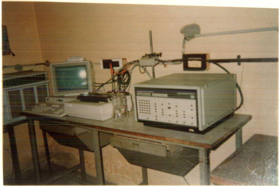
FIG. 2.5 : ELECTROCHEMICAL EXPERIMENTAL SET- UP FOR CORROSION MEASUREMENTS
