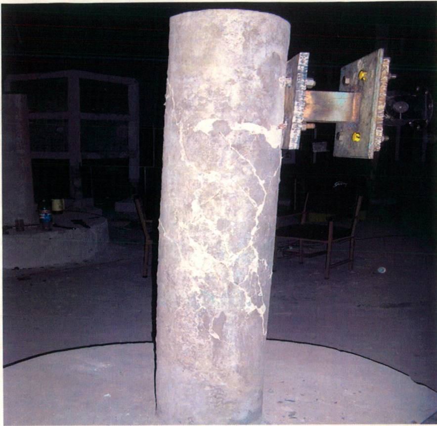
Plate 5.12 Model M2 in Pulling Condition
