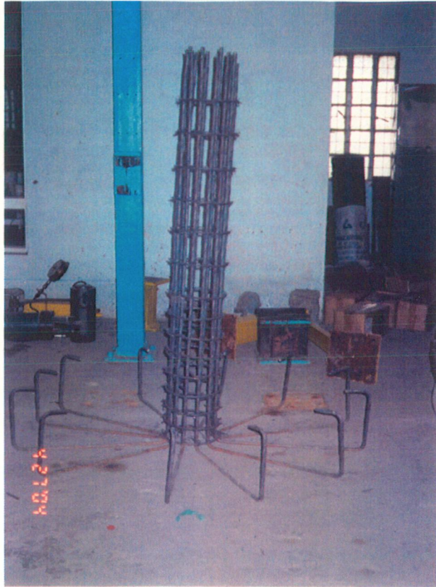
Plate 3.1 Reinforcement Detailing of Models M1 and M2
