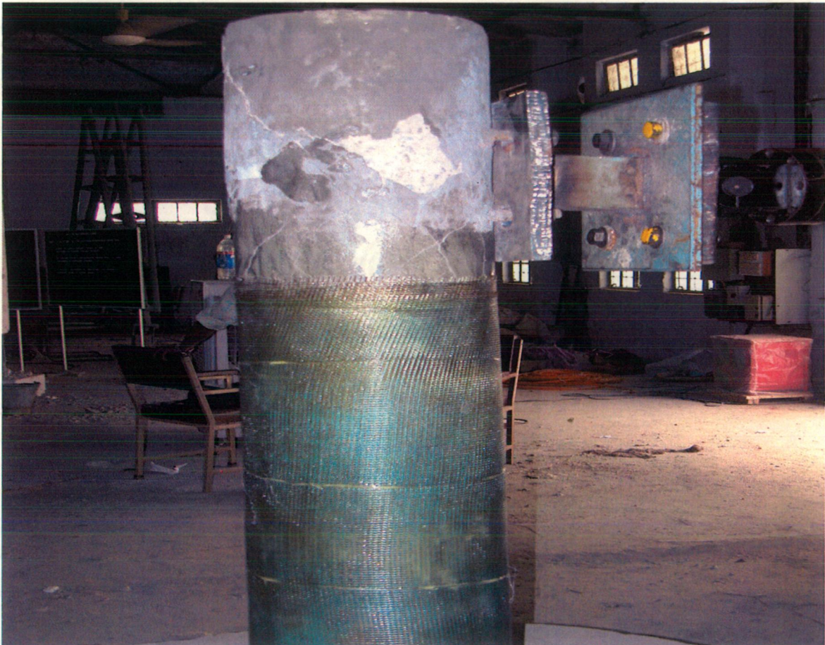
Plate 5.15 Cracks in Model M2
