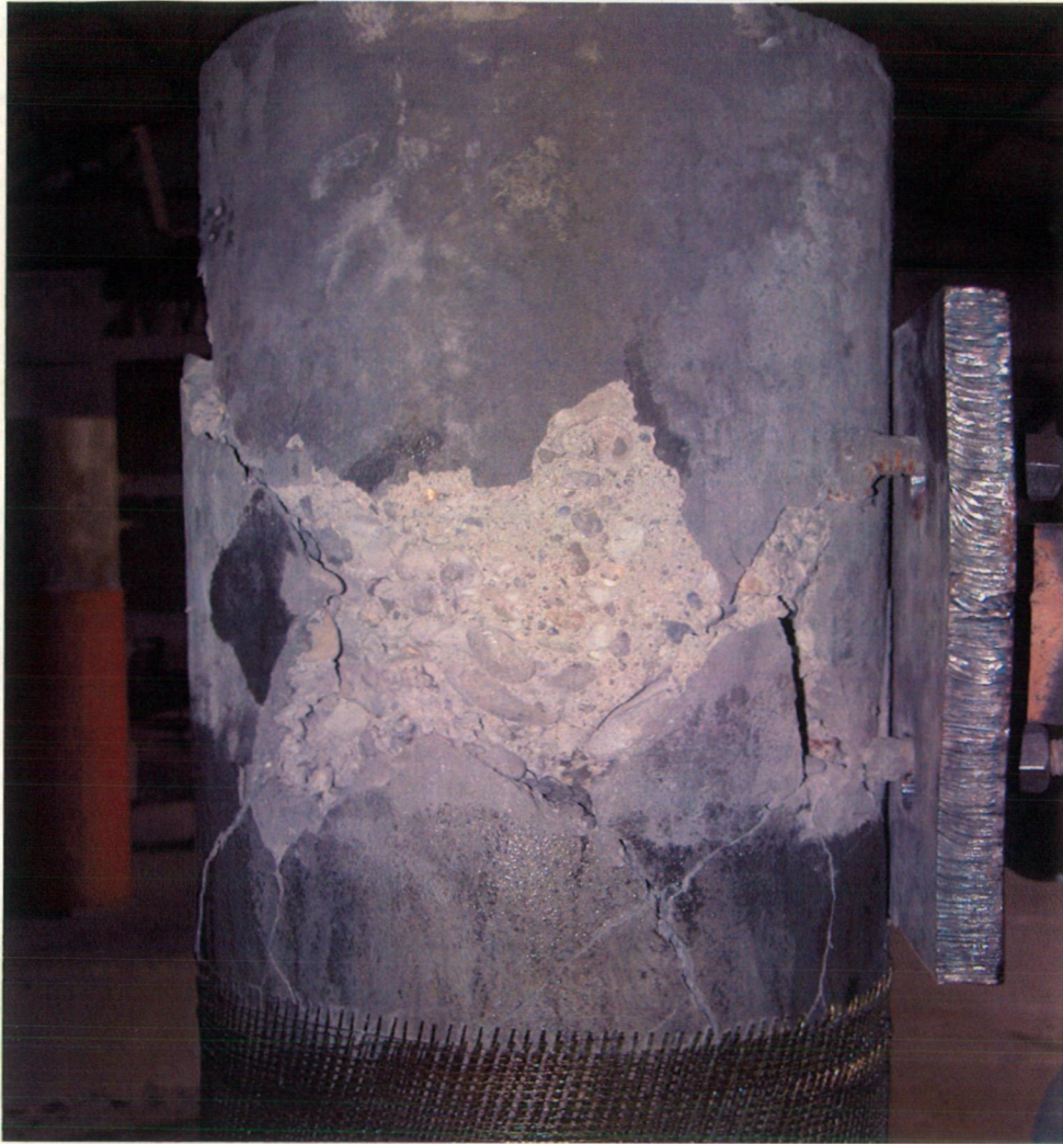
Plate 5.16 Spalling of Concrete at top of the Model M2
