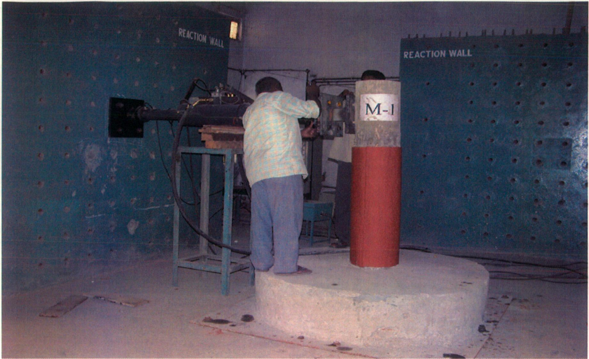
Plate 5.6 Test Set-up of Model M1 after Retrofitting
