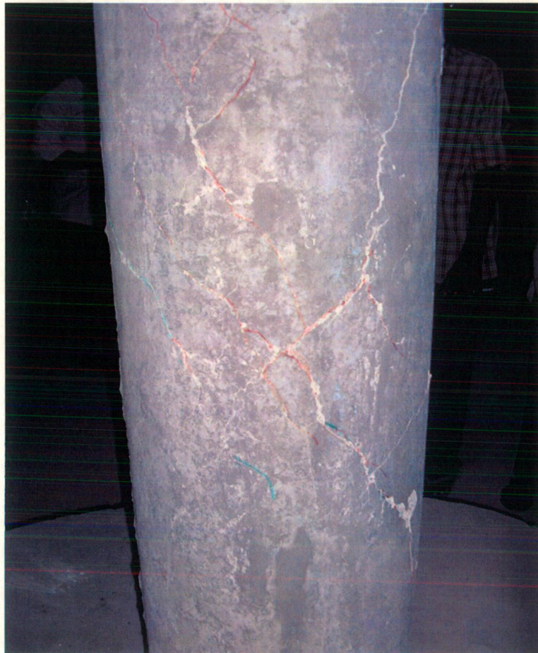
Plate 5.10 Concentric Cracks in Model M1 after Retrofitting
