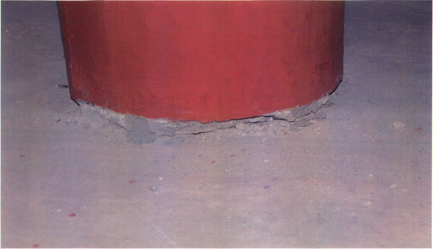
Plate 5.10 Concentric Cracks in Model M1 after Retrofitting
