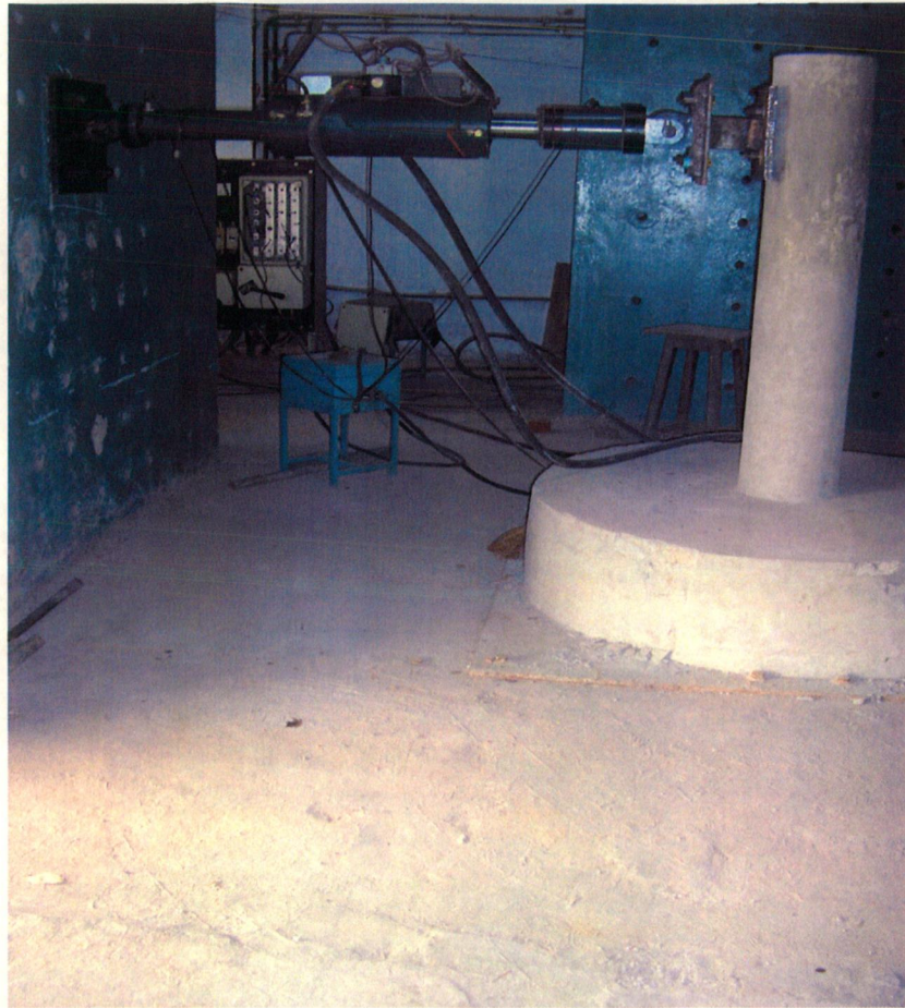
Plate 3.6 Model M1 while Testing (Extreme position of actuator)
