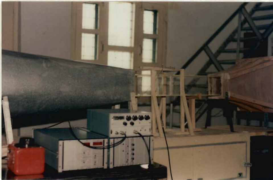
Fig.5.8 Calibration tunnel with instrumentation
