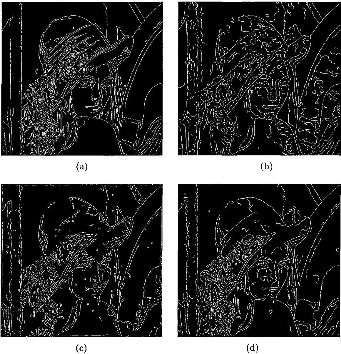
Figure 5.6: Edge profile a) Original b) AWMF filtered c) ARGF filtered d) SRAD filtered
