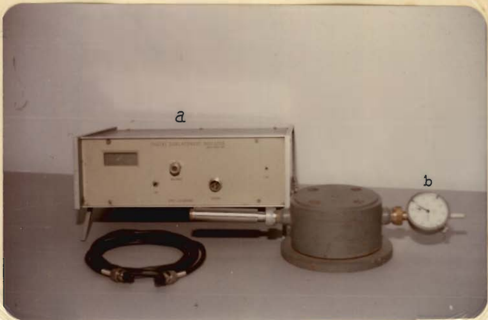
Fig.5.5 - Read-out Units for Use with load Cells a) Electrical Read-out unit b) Dial Gauge
