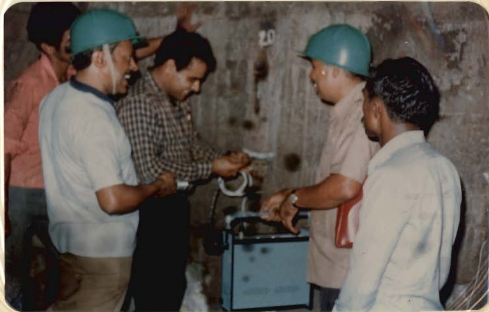
Fig.5.6 - An Electrical Read-out Unit being Used in a Tunnel
