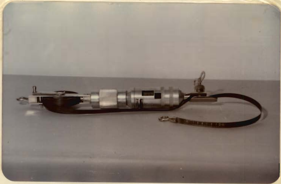
Fig.5.9 - Tape Extensometer Used for Measuring Tunnel Closure
