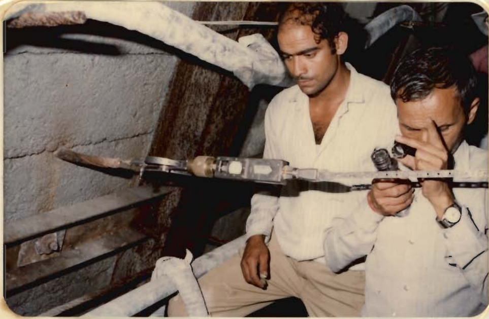
Fig.5.12(a) - A Tape Extensometer Observation Being Taken at a Tunnel Section
