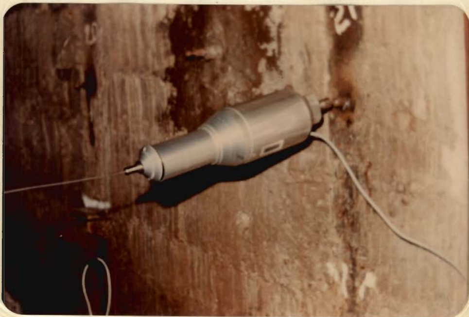
Fig.5.10 - DISTOMAT Used for Measuring Tunnel Closure in Bagur-Navile Tunnel
