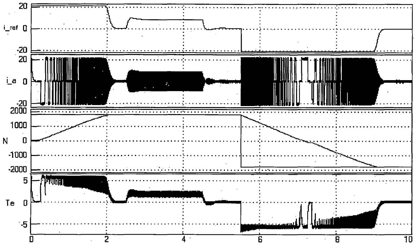
Figure.54. Starting, Speed Reversal and Load Perturbation Response of FSTPI-BLDCM system with PI Speed Controller, capacitance=5000 \mu f and HHH_{initial}=100 or 011. (x-axis is time axis in seconds)
