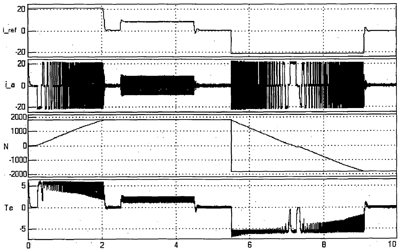
Figure.58. Starting, Speed Reversal and Load Perturbation Response of FSTPI-BLDCM system with fuzzy Speed Controller, capacitance=5000 \mu f and HHH_{initial}=100 or 011. (x-axis is time axis in seconds)
