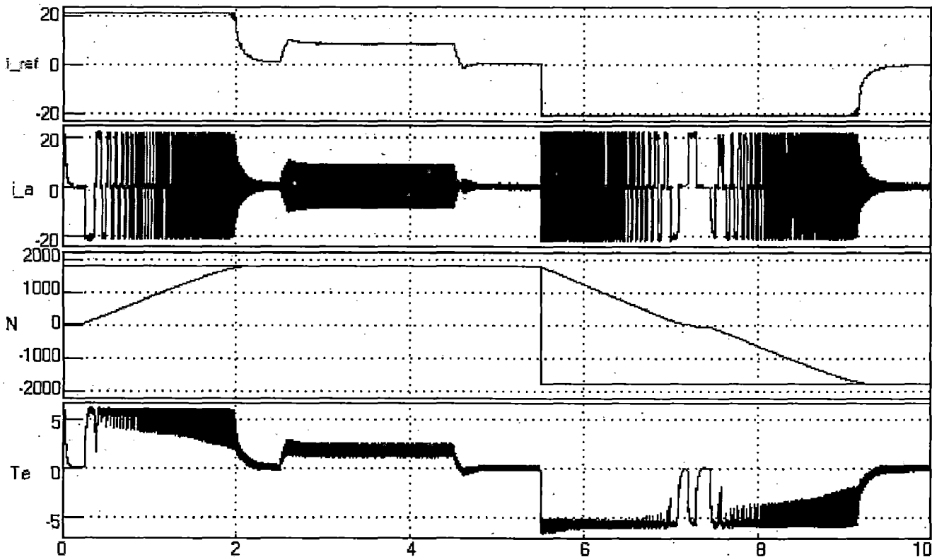
Figure.56. Starting, Speed Reversal and Load Perturbation Response of FSTPI-BLDCM system with sliding mode Speed Controller, capacitance=5000 \mu f and HHH_{initial}=100 or 011. (x-axis is time axis in seconds)
