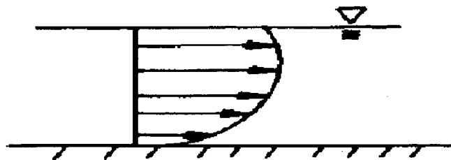
Fig.2.1 Typical Velocity Profile in Open Channel, (Source: www.usgs.com , [25])
