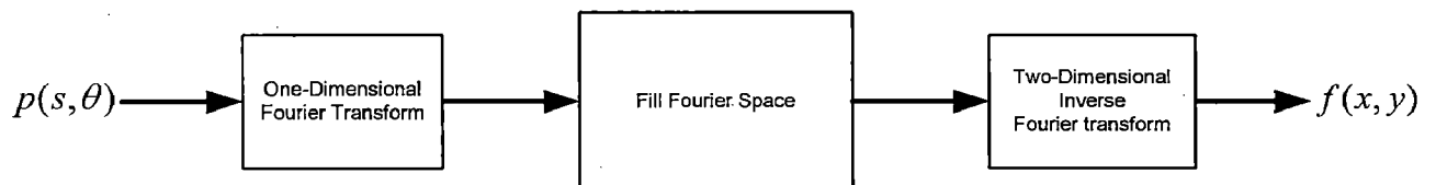
Figure 3.2: A conceptual block diagram of Fourier-based Reconstruction
