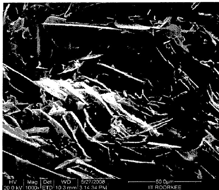
Fig B -3: Scanning electron micrograph of BFA before adsorption at 1000 X Magnification
