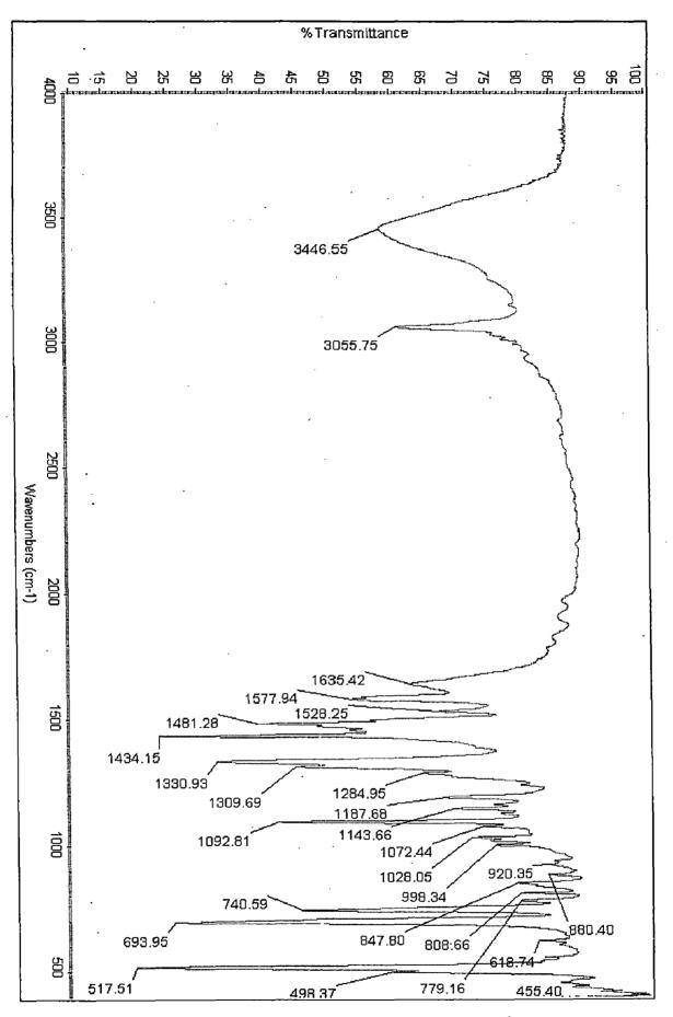
Figure A.6: IR Spectrum of  $Ru(PPh_3)_2L^3Cl$
