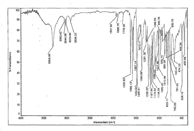
Figure 3.2: IR Spectrum of Ligand  $L^2$
