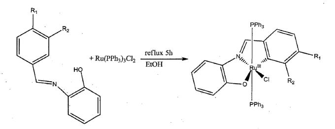
Figure 2.2: Synthesis of  $Ru(PPh_3)_2L^nCl$
