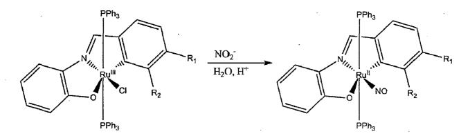
Figure 2.3: Synthesis of  $Ru(PPh_3)_2L^n(NO)$
