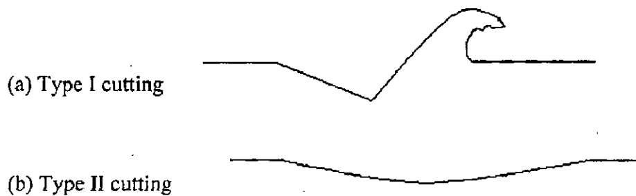
Fig. 2.3 Schematic view of (a) type I cutting by an angular particle, rotating forwards during impact; (b) type II cutting by an angular particle, rotating backwards during impact (Hutchings, 1979).
