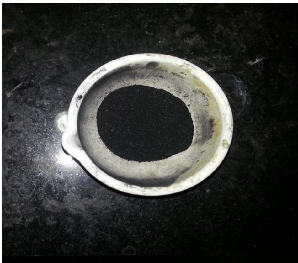
Fig 3.3 Activated corn cob, final product
