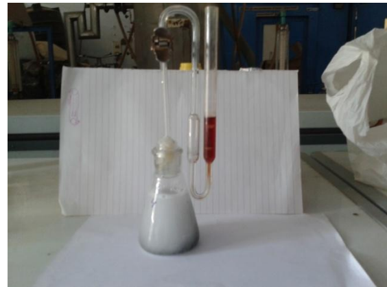
Fig: 3.9 SDDC solution after generation of arsine gas
