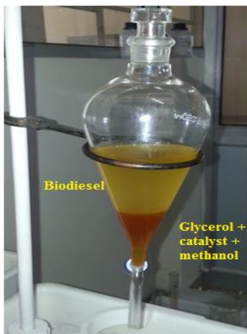
Figure 4.2 Phase separation of reaction product
