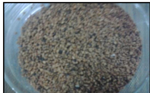
Laterite after acid base treatment(500-1000) microns
