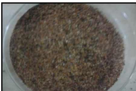
Laterite after acid base treatment(350-500) microns
